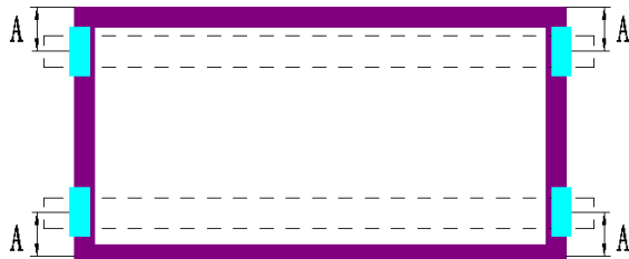
Use 4 clamps on the short side. Mounting rails run parallel to the long side frame.
