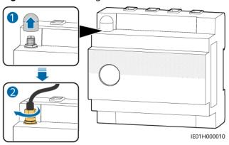
Figure 5-15 Installing a WLAN antenna
