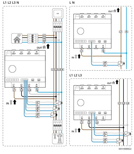
Figure 5-8 External CT connection (current > 63 A)
