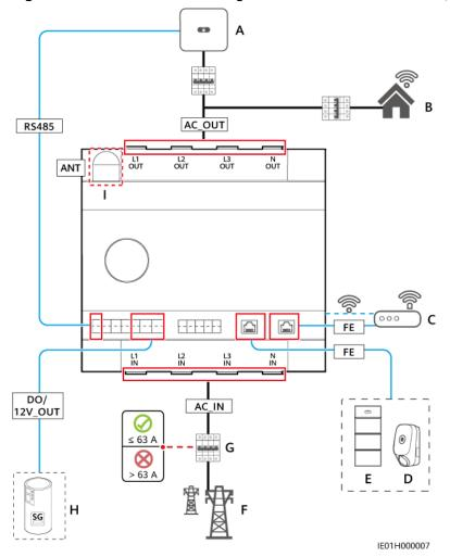
**Figure 5-1** Cable connection diagram: internal CT connection (current  $\leq$  63 A)
