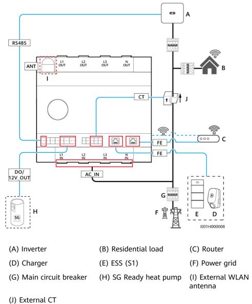
Figure 5-2 Cable connection diagram: external CT connection (current > 63 A)
