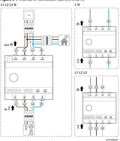
Figure 5-7 Internal CT connection (current  $\leq$  63 A)
