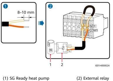
Figure 5-11 Connecting the power DO to the SG Ready heat pump
