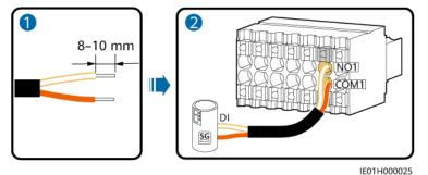
Step 3 Insert the 14-pin signal connector into the EMMA.
