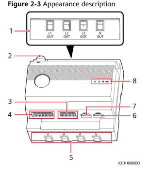
(1) AC output port (L1 OUT/L2 OUT/L3 OUT/N OUT) (ANT) (3) 12 V input/RS485 communication/ external CT input port (12V\_IN/ RS485/CT Input) V\_OUT/DO)
