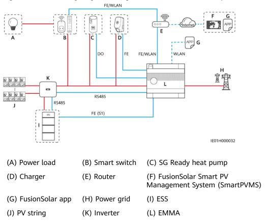
Figure 2-2 Networking diagram (using the EMMA-A02 as an example)
