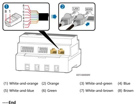
Figure 5-14 Connecting FE communications cables
