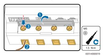
**Step 3** Connect all AC power cables and external CT cables based on the power grid connection.
