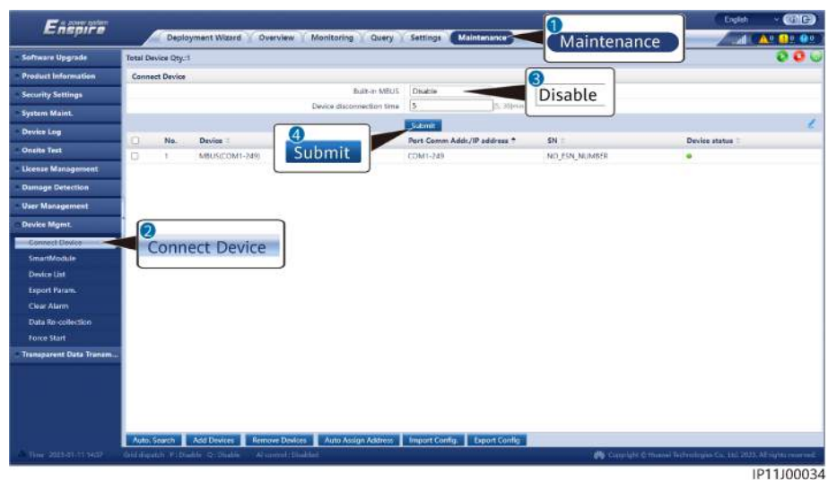
Figure 6-47 Setting parameters for a built-in MBUS module
