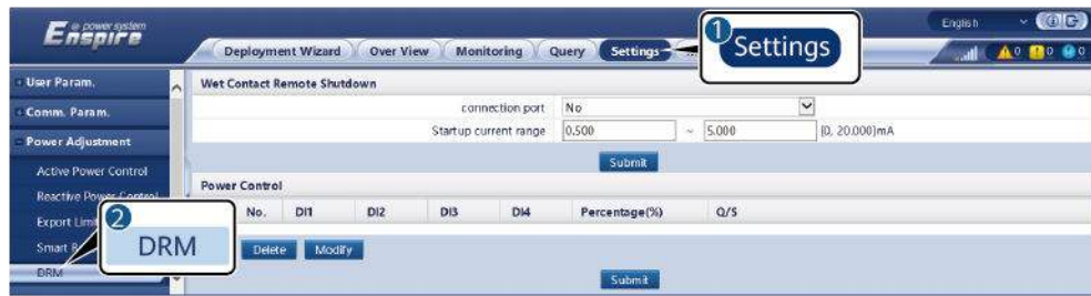
Figure 6-78 Setting DRM parameters
