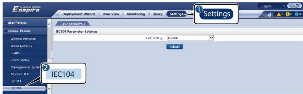
Figure 6-39 Setting IEC 104 parameters
