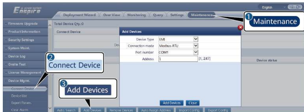
Figure 6-57 Setting access parameters
