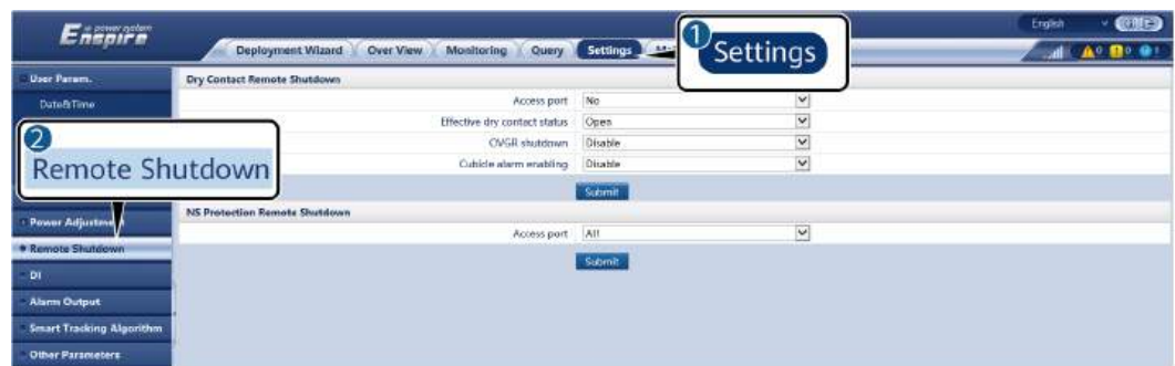
Figure 6-80 Dry contact remote shutdown
