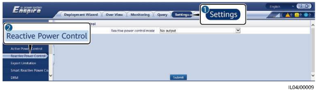
Figure 6-70 Reactive power control
