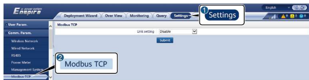
Figure 6-38 Setting Modbus TCP parameters
