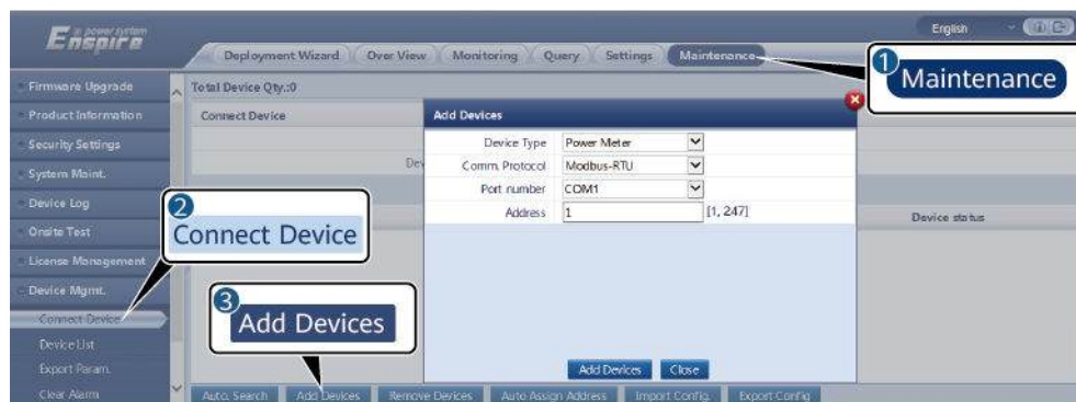
Figure 6-56 Setting access parameters
