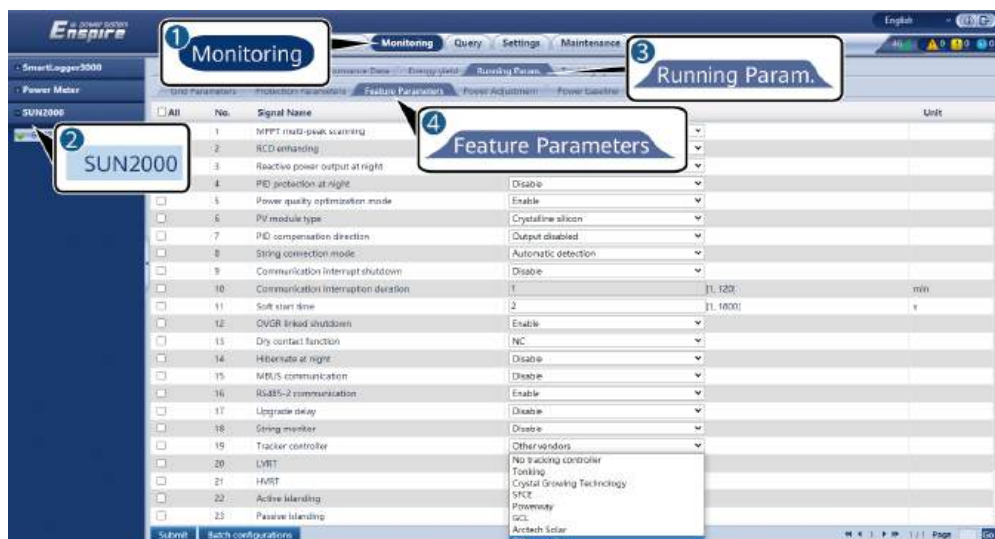
Figure 6-50 Setting tracking system controller
