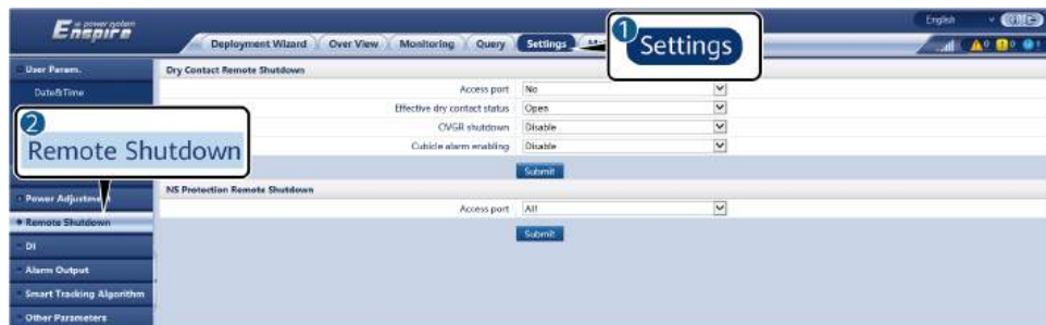
Figure 6-82 NS protection remote shutdown
