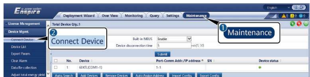
Figure 6-43 Setting parameters for a built-in MBUS module
