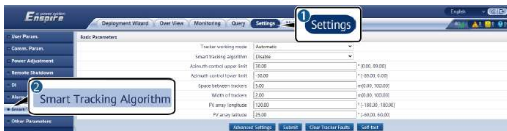
Figure 6-64 Smart tracking algorithm (SDS) parameters
