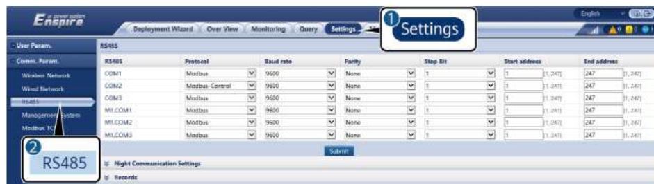
Figure 6-83 Setting RS485 parameters
