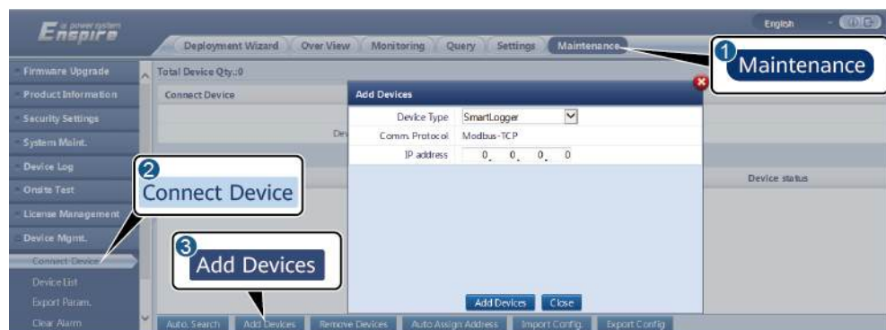
Figure 6-42 Setting access parameters
