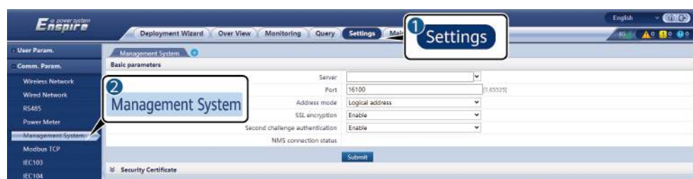
Figure 6-32 Setting management system parameters
