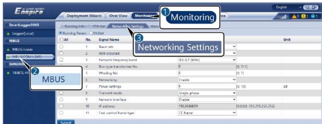
Figure 6-46 Setting external MBUS networking
