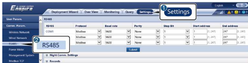
Figure 6-40 Setting RS485 parameters
