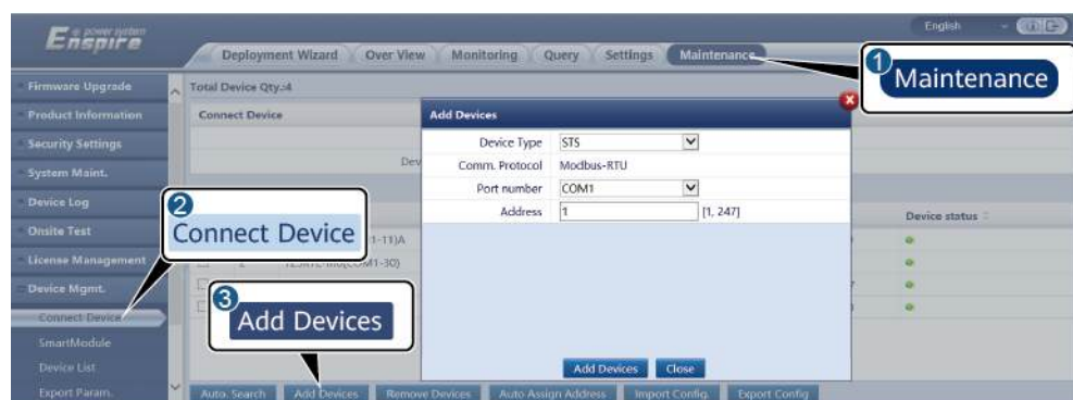
Figure 6-59 Setting access parameters
