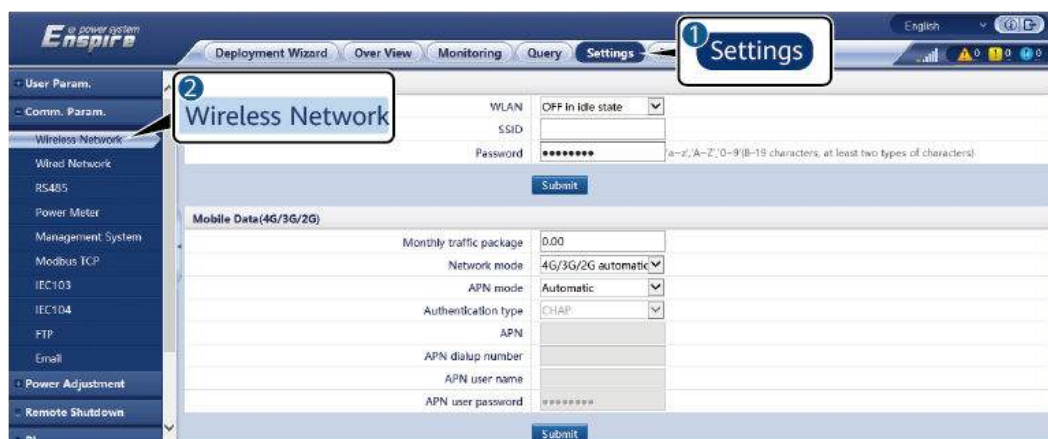
Figure 6-30 Setting mobile data parameters
