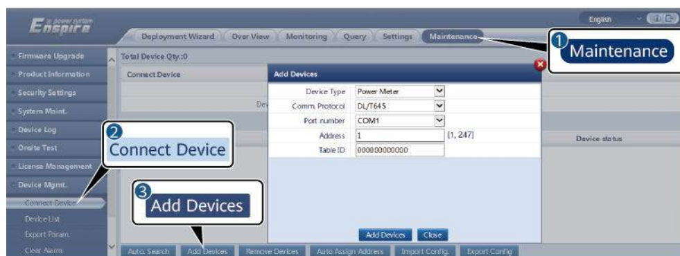
Figure 6-55 Setting access parameters
