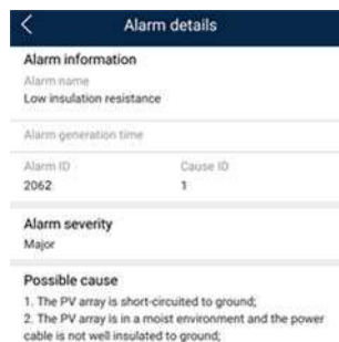
Figure D-1 Alarm details
