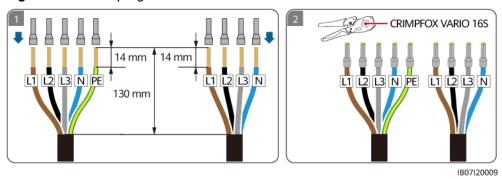
**Step 4** Connect the inverter AC input power cables.
