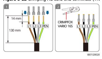
**Step 2** Connect the non-backup load output power cable.
