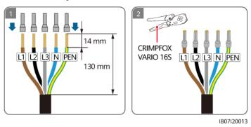
**Figure 5-16** Crimping AC cord end terminals for the SmartGuard-63A-AUT0 (TN-S/TN-C-S/TT system)
