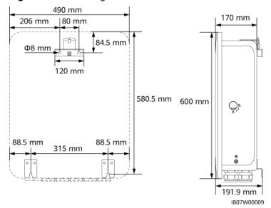
Figure 4-1 Mounting bracket dimensions
