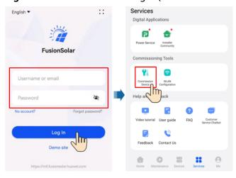
**Step 2** Connect to the inverter WLAN, log in as **Installer**, and access the device commissioning screen.
