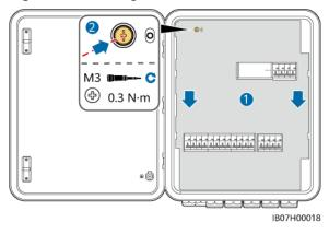
**Step 2** Remove the bypass switch latch and turn on the bypass switch.
