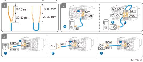
Figure 5-30 Connecting the signal cable to the 14-pin terminal
