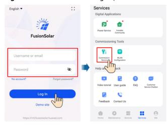
**Step 2** Connect to the SmartAssistant WLAN, log in as **Installer**, and access the device commissioning screen.
