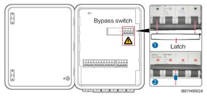
**Step 3** Turn on the four switches shown in the following figure (using the connection to three parallel MAPO inverters as an example).
