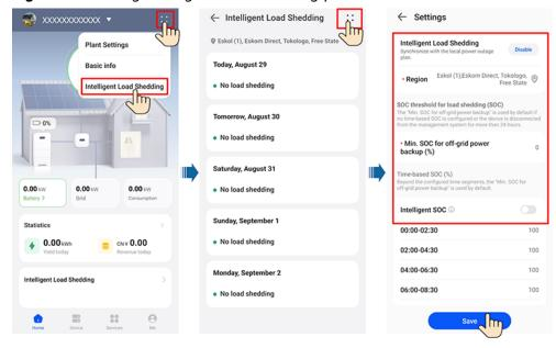
Figure F-1 Setting intelligent load shedding parameters
