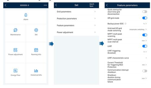
Figure 6-11 Setting off-grid mode
