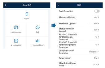
Figure 6-14 Setting generator parameters
