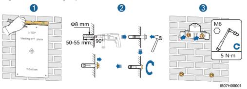
**Step 3** Install the SmartGuard on the mounting bracket and tighten the nuts.
