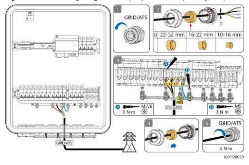
Figure 5-11 Connecting the grid AC output power cable (TN-C system)
