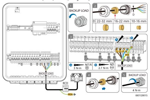
**Figure 5-19** Connecting the backup load output power cable of the SmartGuard-63A-AUT0 (TN-S/TN-C-S/TT system)
