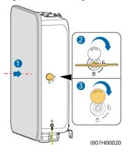
Figure 6-8 Closing the maintenance compartment
