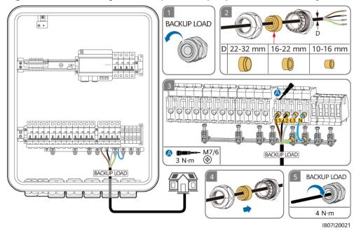
Figure 5-20 Connecting the backup load output power cable (TN-C system)
