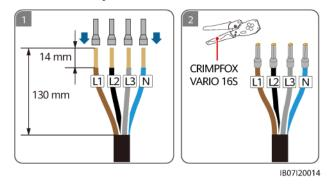
Figure 5-17 Crimping AC cord end terminals (TN-C system)
