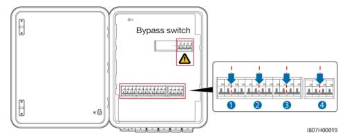
2. Remove the bypass switch latch, turn on the bypass switch, and then turn on switches 3 and 4 shown in the figure.
