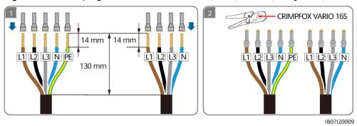
Figure 5-22 Crimping AC cord end terminals (TN-C system)
