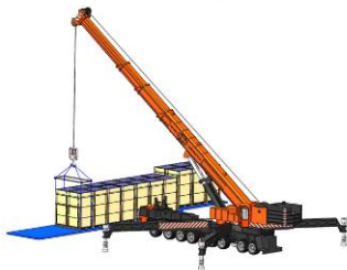
Long-side vertical package unloading with crane
