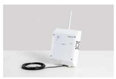
The mutual communication of the units takes place wirelessly on the frequency 433 MHz, which is for increased reliability two-way, quality data is transmitted several times per second connection and operating states of both units. In case of communication failure, both the units go to the defined safe state.
