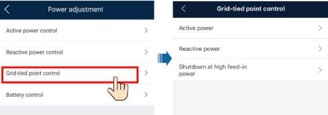
Figure 7-10 Grid-tied point control
