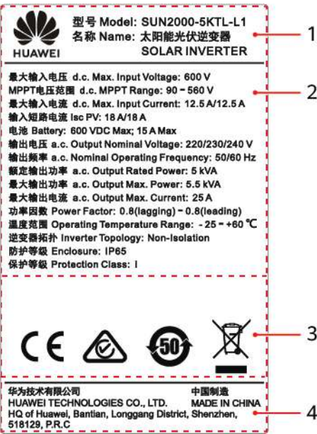
Figure 2-7 Nameplate (using SUN2000-5KTL-L1 as an example)
