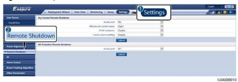
Description **Parameter** Set the parameter to Al1 port connected to Al Access port signals. The SmartLogger shuts down the inverter over the voltage change detected at the AI1 port.
