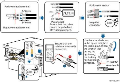
Figure 5-13 Connecting DC power cables
