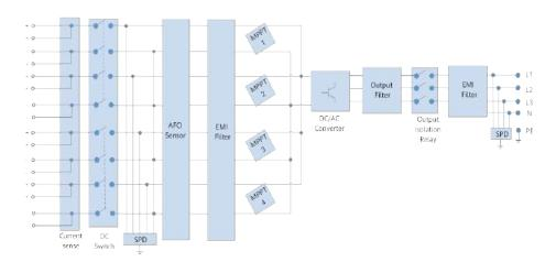
Figure 2-5 Schematic diagram
