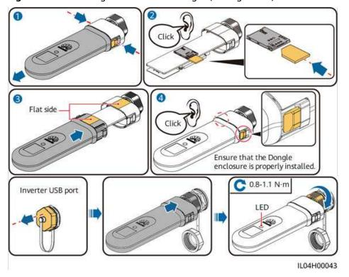
• WLAN-FE Smart Dongle (WLAN communication)
