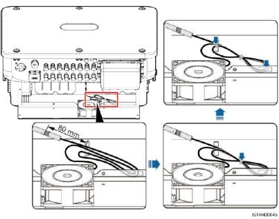
Figure 8-5 Binding a cable
