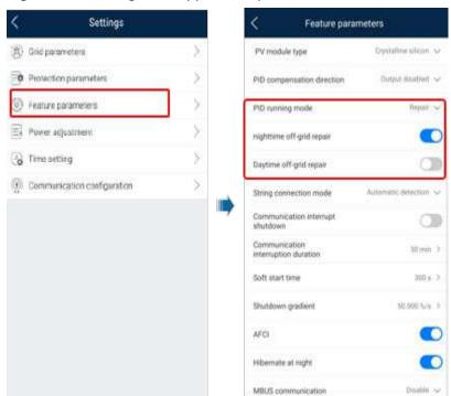
Figure C-1 Setting PID suppression parameters
