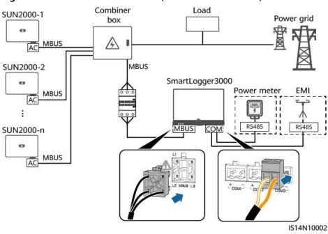
Figure 5-23 MBUS communication (C&I scenario in China)
