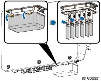
**Step 2** Connect the AC output power cable.
