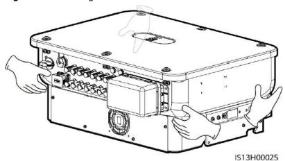
Figure 4-10 Moving the inverter
