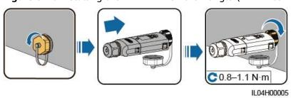
• WLAN-FE Smart Dongle (FE communication)
