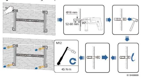
Figure 4-15 Installing an expansion bolt
