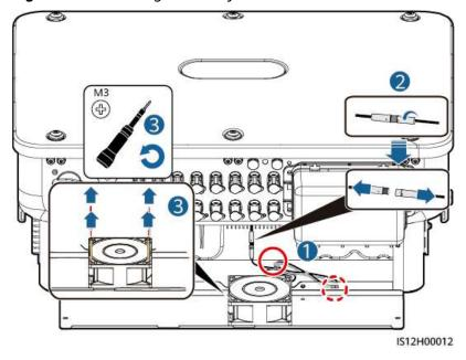
Figure 8-4 Removing the faulty fan
