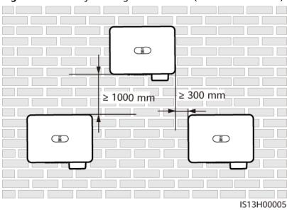
Figure 4-4 Two-layer triangle installation (not recommended)
