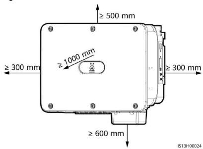
• If multiple inverters need to be installed, horizontal installation, stacked installation on supports, and back-to-back staggered installation on supports are recommended. Triangle installation, stacked installation on a wall, and back-to-back installation on supports for multiple inverters are not recommended.
