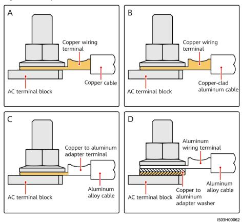
Figure 5-4 Requirements for the OT/DT terminal
