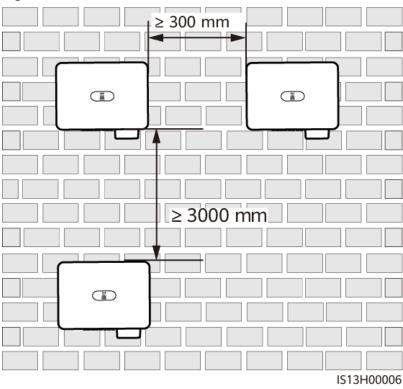
Figure 4-6 Stacked installation on a wall (not recommended)
