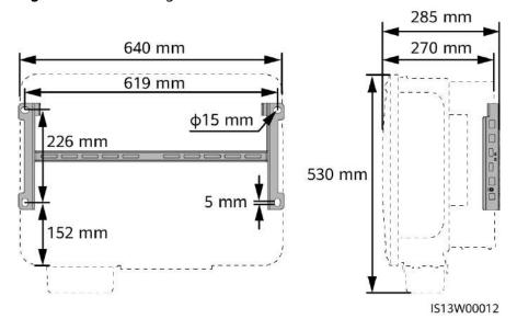
Figure 4-12 Mounting bracket dimensions
