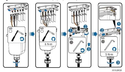
Figure 5-11 Wiring requirements
