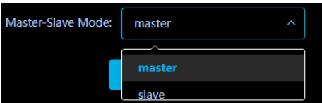
Fig 31 Set the RS485 master/slave mode
