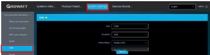
Fig 37 Set the CAN protocol type
