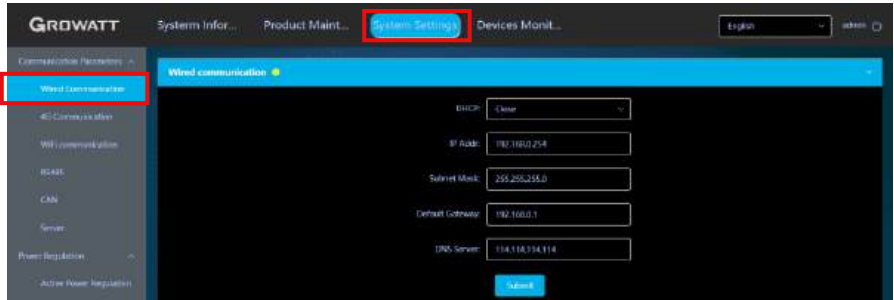
Fig 83 Disable the DHCP function
