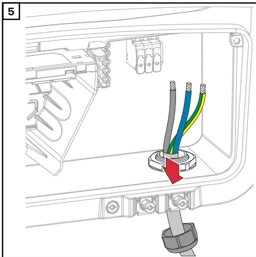
Remove the mains cable from the inverter.
