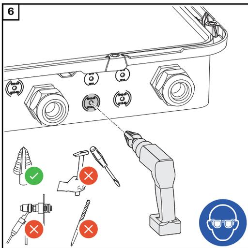
Drill out the optional cable bushing with a step drill.
