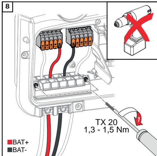
Fasten the screws of the cable guide to the housing using a screwdriver (TX20) and a torque of 1.3 - 1.5 Nm.
