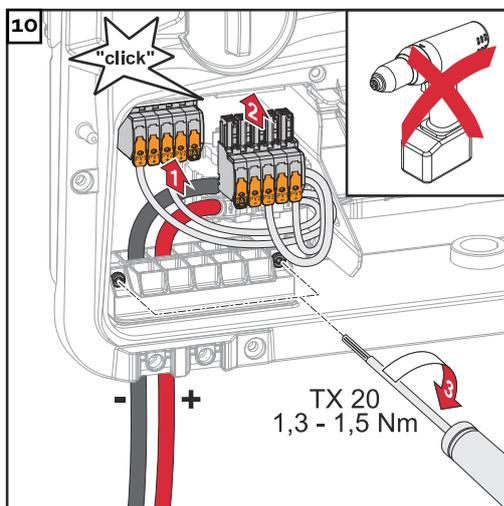
Insert the DC terminals into the respective slot until they engage. Fasten the screws of the strain-relief device to the housing using a screwdriver (TX20) and a torque of 1.3-1.5 Nm.
