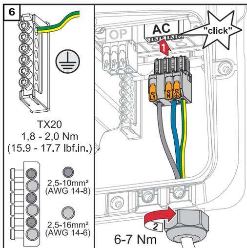
Insert the AC terminal into the AC slot until it engages. Fasten the union nut of the cable gland with a torque of 6 - 7 Nm.
