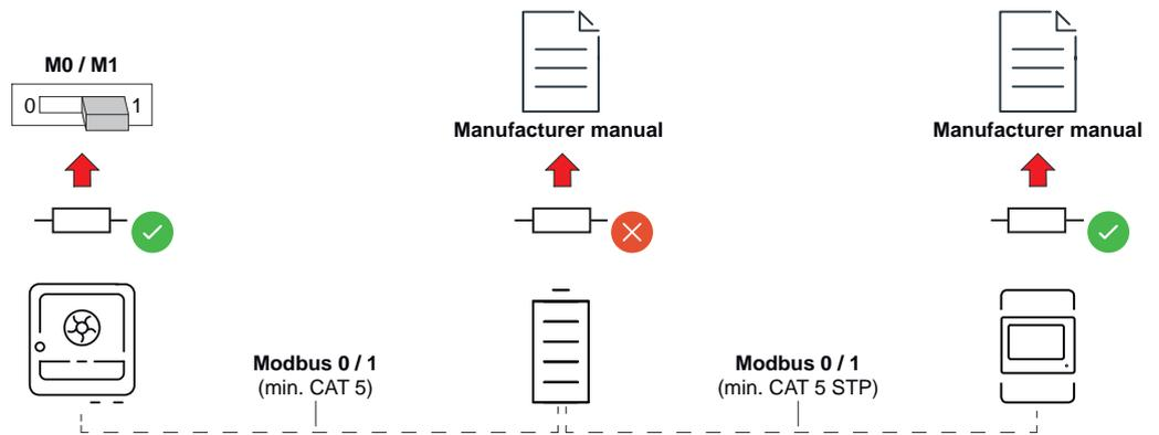
**Installing the WSD (wired shutdown)**
