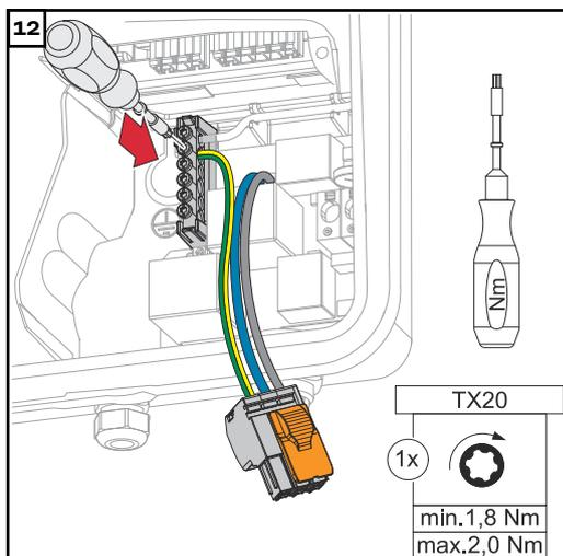
Fasten the PEN conductor to the second input of the ground electrode terminal from the top using a screwdriver (TX20) and a torque of 1.8-2 Nm.
