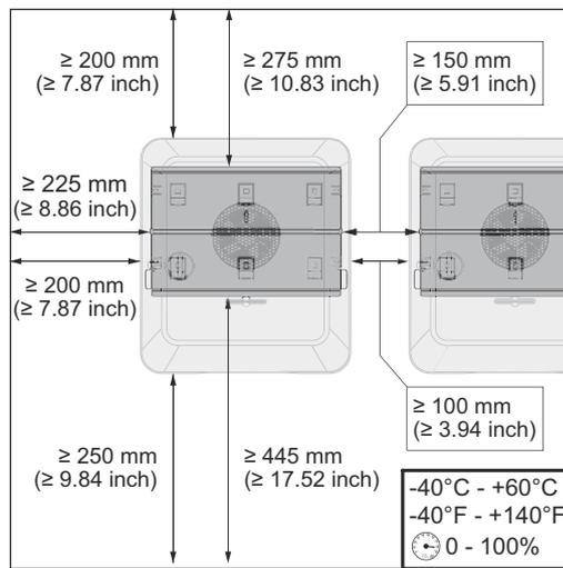
Only install on a solid, non-flammable surface.
