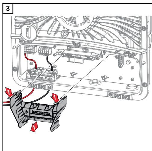
Remove the connection area divider by pressing the snap tabs.
