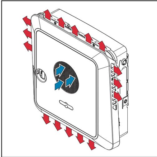
Ambient air is drawn in at the front of the device by the fan and blown out at the sides. The even heat dissipation allows several inverters to be installed next to each another.
