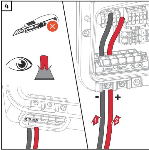
Manually push the DC cables through the DC bushings.
