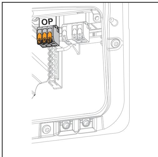
With the PV Point, in the event of a failure of the public grid, 1-phase electrical devices can be connected to the Opportunity Power (OP) terminal and supplied with a maximum power of 3 kW, if enough power is available from the PV modules or an optional battery. In grid-connected operation, the OP terminal is not supplied with voltage, therefore the connected loads will not be continuously supplied with power.
