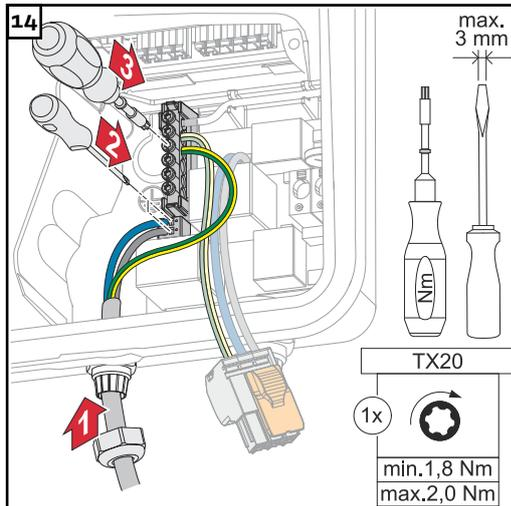
Connect the phase/neutral conductors to the terminals provided. Fasten the ground conductor to the third input of the ground electrode terminal from the top using a screwdriver (TX20) and a torque of 1.8-2 Nm.
