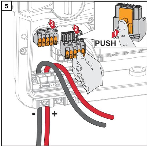
Press the lock on the back of the terminal and pull off the DC terminals.
