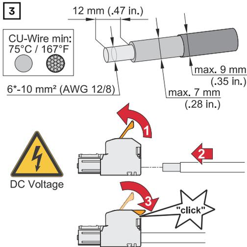
\* See the battery manufacturer's operating instructions for the minimum cable cross-section.
