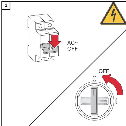
Switch off power to the inverter and wait for the specified time until the capacitors have discharged and the fan has shut down. Turn the DC disconnector to the "Off" switch setting.
