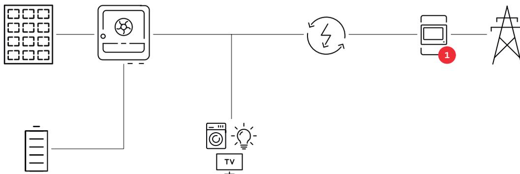
**Operating mode – Inverter with battery, Ohmpilot, and backup power function**
