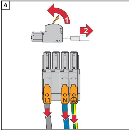
Disconnect the single conductors from the AC terminal (only necessary if the installation already exists).
