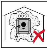
The inverter is essentially designed to be dustproof (IP 66). In areas of high dust accumulation, dust deposits may collect on the cooling surfaces, and thus impair the thermal performance. Regular cleaning is required in this case; see the chapter headed [Operation in dusty environments](#) on page 177. We therefore recommend not installing the inverter in areas and environments with high dust accumulation.
