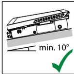
The inverter is suitable for installation on a sloping surface (min. slope of underside 10°).
