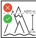
The inverter must not be installed or operated at more than 4,000 m above sea level.
