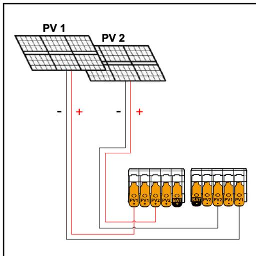
PV 1 less than or equal to 41.25 A ( $I_{SC PV1}$ )
