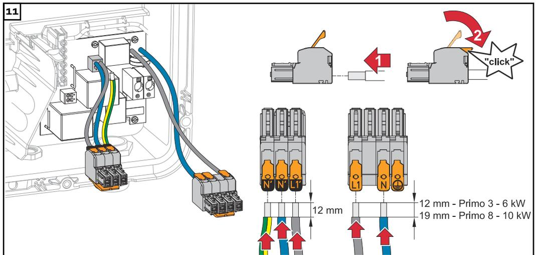
Strip the single conductors (Primo 3 - 6 kW = 12 mm, Primo 8 - 10 kW = 19 mm). Lift to open the AC terminal's operating lever and insert the stripped single conductor into the slot provided, all the way up to the stop. Then close the operating lever until it engages.
