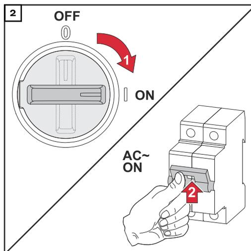
Set the DC disconnect to the "on" switch position. Turn on the automatic circuit breaker.
