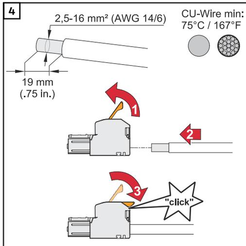
Strip the insulation of the single conductors by 19 mm. Select the cable cross-section in accordance with the instructions in [Permissible cables for the electrical connection](#) from page 65. Lift to open the terminal's operating lever and insert the stripped single conductor into the slot provided as far as it will go. Then close the operating lever until it engages.
