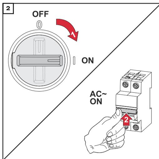
Set the DC disconnecter to the "on" switch position. Turn on the automatic circuit breaker.
