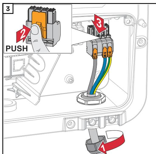
Press the lock on the back of the terminal and remove the AC terminals. Loosen the cable gland.
