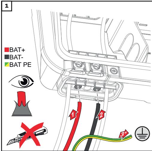
Push the battery cables through the DC bushings by hand.
