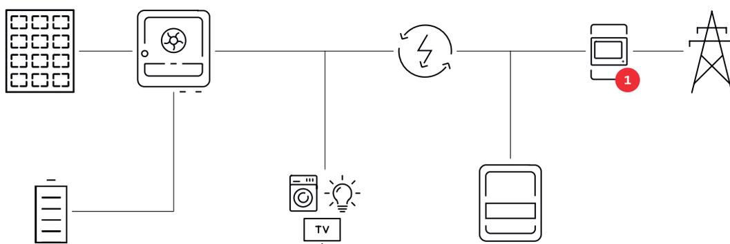
**Operating mode – Inverter with battery, another inverter, and backup power function**
