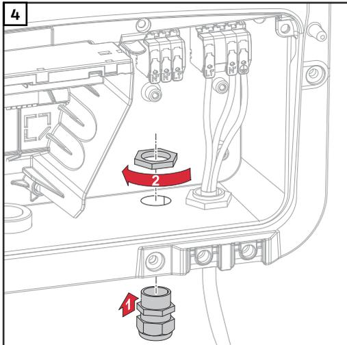
Insert the cable gland into the hole and secure to the torque specified by the manufacturer.
