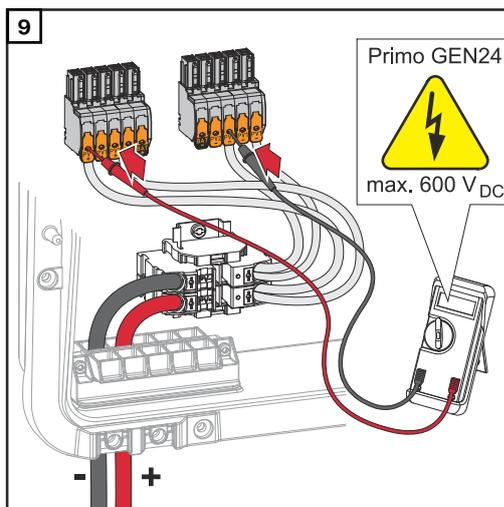
Use a suitable measuring instrument to check the voltage and polarity of the DC cabling.
