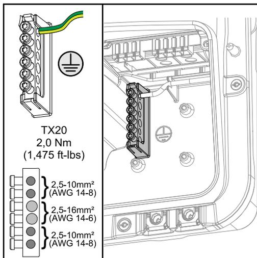
The ground electrode terminal  $\oplus$  allows additional components to be earthed, such as:
