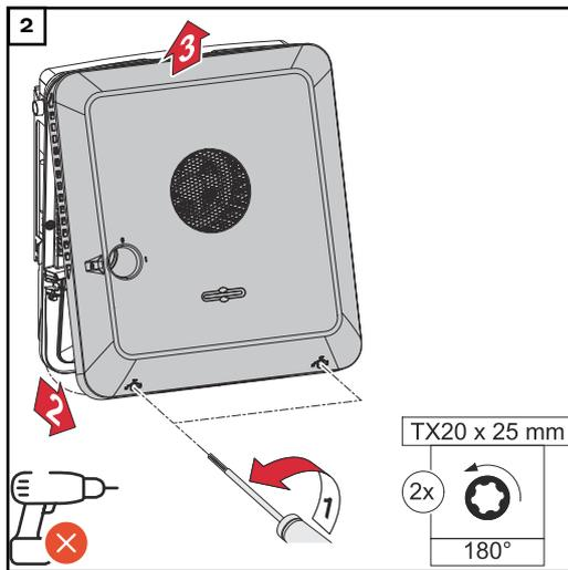
Loosen the screws on the underside of the housing cover by rotating them 180° to the left using a screwdriver (TX20). Then lift the housing cover away from the inverter at the bottom and detach from above.
