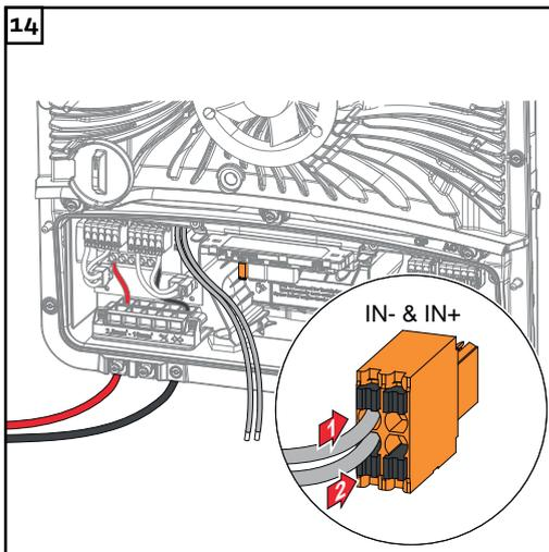
Connect the signal cable to the push-in WSD terminal on the IN- and IN+ slots, observing the labeling.
