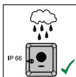
The inverter is suitable for outdoor installation.
