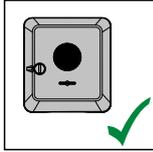
The inverter is suitable for vertical installation on a vertical wall or column.
