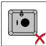
Do not install the inverter in a horizontal position on a vertical wall or column.
