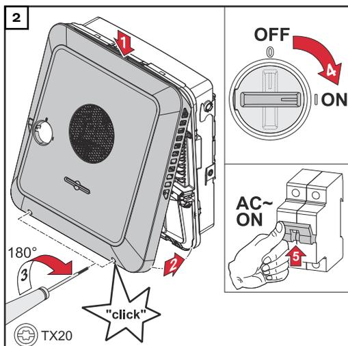
Clip the housing cover in at the top of the inverter.
