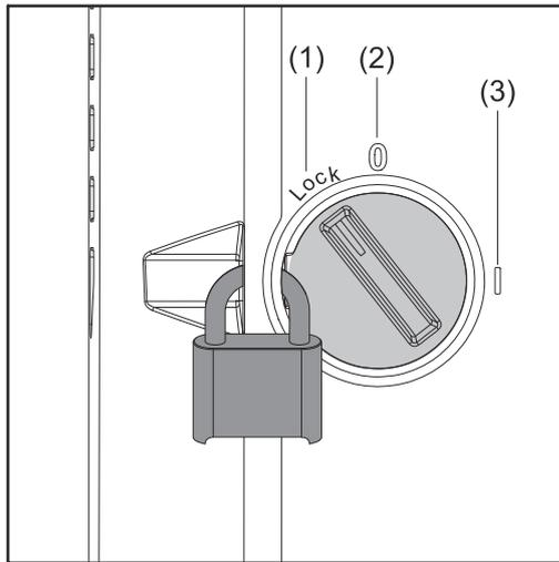
The DC disconnect has three switch settings:
