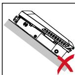
Do not install the inverter on a sloping surface with the connections upwards.
