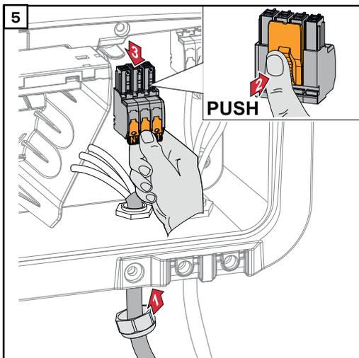
Guide the mains cable through the cable gland from below. Pull off the OP terminal.
