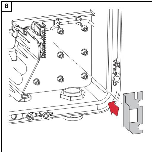
Insert the insulating film on the right side of the ground electrode terminal.
