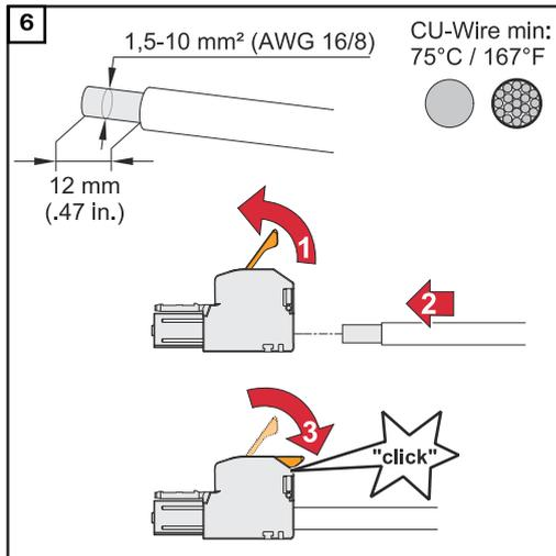
Strip the insulation of the single conductors by 12 mm. The cable cross-section must be between 1.5 mm<sup>2</sup> and 10 mm<sup>2</sup>. Lift to open the terminal's operating lever and insert the stripped single conductor into the slot provided, all the way up to the stop. Then close the operating lever until it engages.
