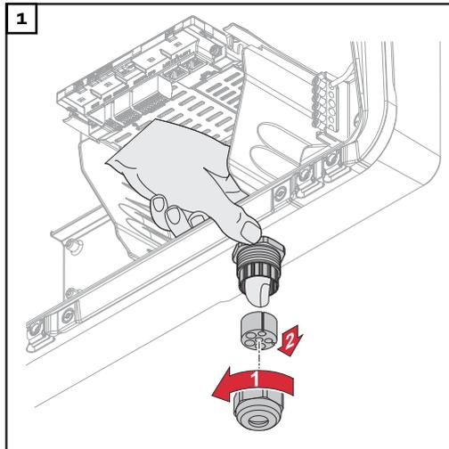
Undo the cable gland union nut and push out the sealing ring and the blanking plug from the inside of the device.
