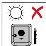
In order to keep inverter heating as low as possible, do not expose the inverter to direct sunlight.
