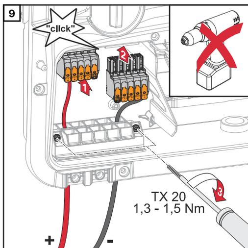
Insert the DC terminals into the respective slot until they engage. Fasten the screws of the cable guide to the housing using a screwdriver (TX20) and a torque of 1.3 - 1.5 Nm.
