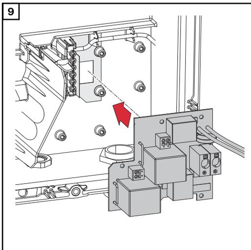
Insert the PC board into the inverter.
