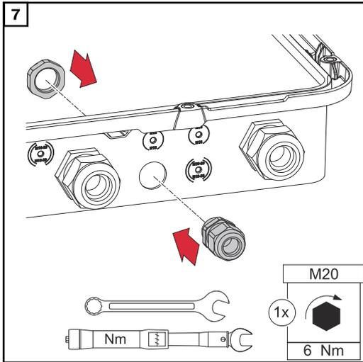
Insert the cable gland into the hole and tighten to a torque of 6 Nm.
