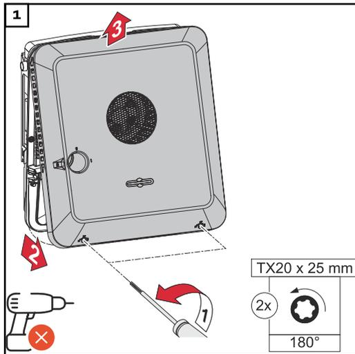
Loosen the two screws on the underside of the housing cover by rotating them 180° to the left using a screwdriver (TX20). Then lift the housing cover away from the inverter at the bottom and detach from above.
