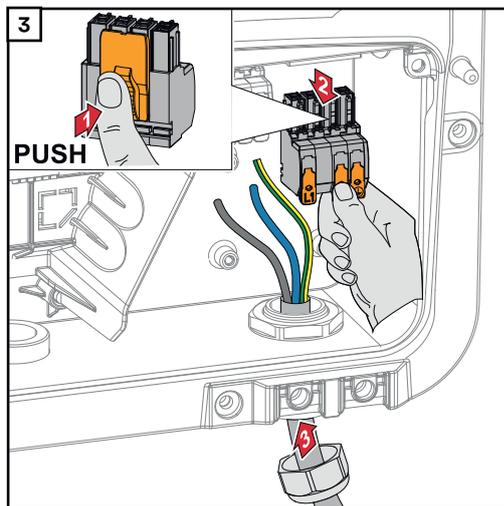
Press the lock on the back of the terminal and remove the AC terminal. Guide the mains cable from below through the cable gland on the right side.
