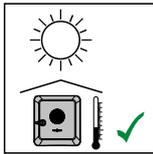
The inverter should be installed in a protected location, e.g., near the PV modules or under an overhanging roof.
