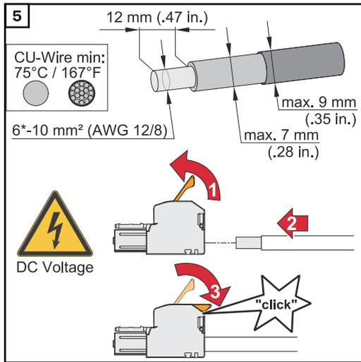
Select the cable cross-section in accordance with the instructions in [Permissible cables for the electrical connection](#) from page 65.
