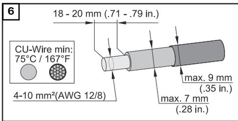
Strip the insulation of the single conductors by 18-20 mm. Select the cable cross-section in accordance with the instructions in [Permissible cables for the electrical connection](#) from page 65.
