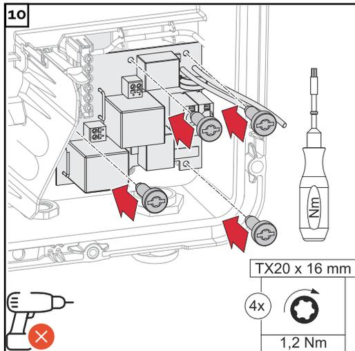
Fasten the PC board with the four screws (TX20) supplied and tighten to a torque of 1.2 Nm.
