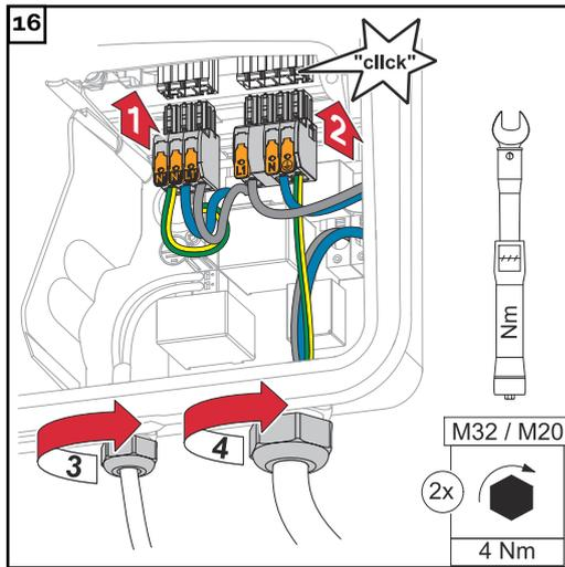
Insert the terminals into the respective slot until they engage. Fasten the union nuts of the cable glands to a torque of 4 Nm.
