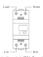
The Ingress Protection rate is IP51, So meter must be installed in door. The whole installation chart shows as below:
