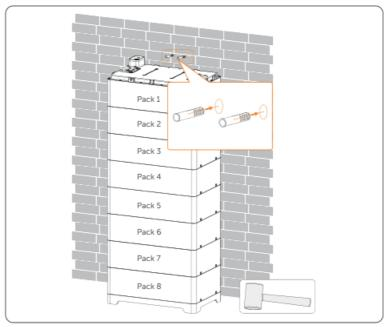
Figure 7-12 Inserting expansion bolt
