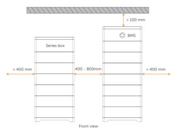
Figure 4-3 Installation clearance for two towers
