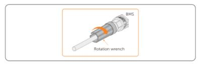
Figure 6-30 Closing communication cable
