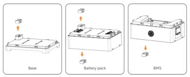
Figure 6-2 Removing dust cover
