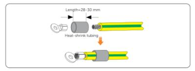
Figure 6-18 Cutting heat-shrink tubing
