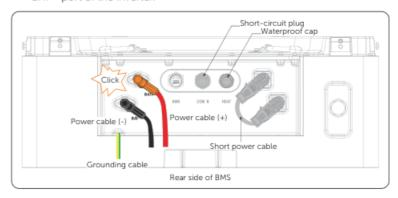
Figure 6-27 Plugging power cables
