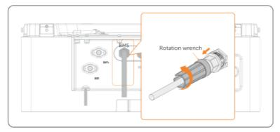
Figure 11-5 Unplugging communication cable
