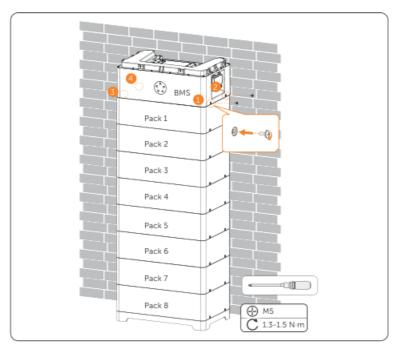
Figure 6-15 Tightening M5 screw
