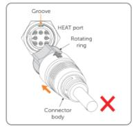
Figure 7-34 Plugging heater cable
