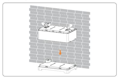
Figure 7-6 Placing battery pack
