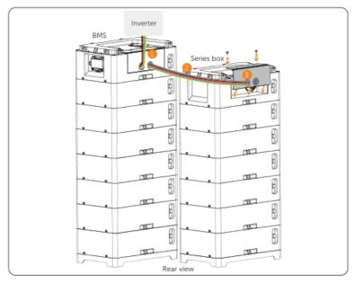
Figure 7-41 Pulling cables and securing cover
