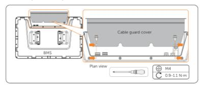
Figure 7-40 Tightening M4 screw
