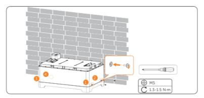
Figure 6-7 Tightening screw
