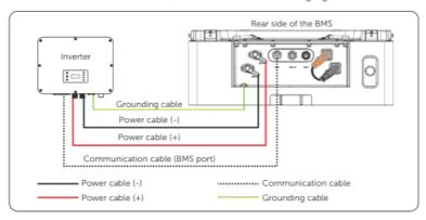
Figure 6-16 Wiring diagram
