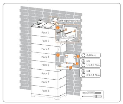
Figure 6-13 Securing assembled bracket
