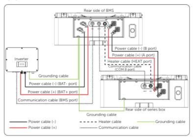
Figure 7-17 Wiring diagram
