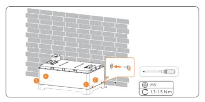
Figure 7-7 Tightening screw
