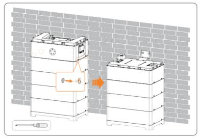
Figure 9-10 Removing BMS
