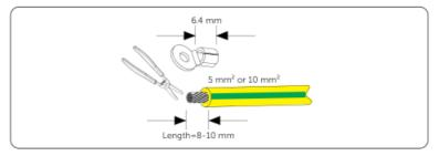
Figure 7-18 Striping cable jacket
