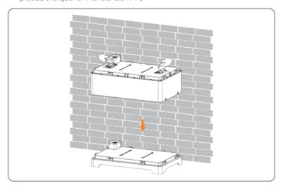
Figure 6-6 Placing battery pack
