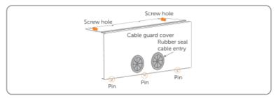
Figure 6-25 Details of cable guard cover
