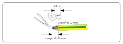
Figure 6-17 Striping cable jacket
