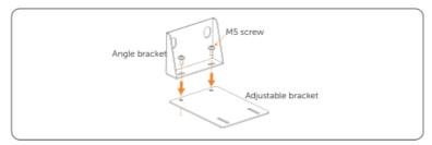
Figure 7-9 Assembling bracket
