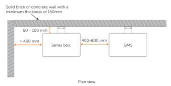
Figure 4-4 Installation clearance for two towers
