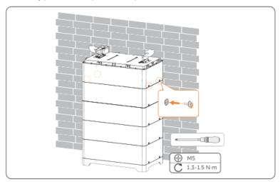
Figure 9-12 Placing battery pack and securing M5 screw
