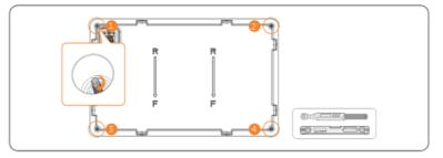
Figure 7-4 Rotating adjustable screw
