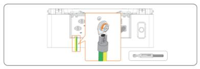
Figure 11-6 Disassembling grounding cable
