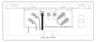
Figure 6-29 Plugging communication cable
