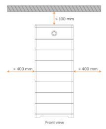
Figure 4-2 Installation clearance for one tower
