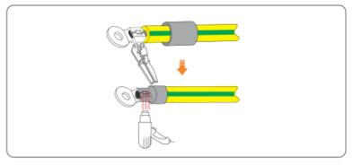
Figure 7-20 Crimping and heating
