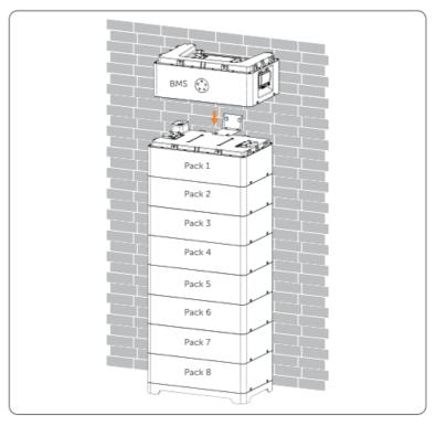
Figure 7-14 Placing BMS
