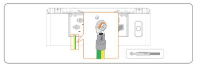
Figure 9-9 Disassembling grounding cable
