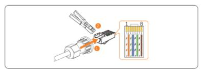
Figure 6-23 Crimping RJ45
