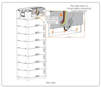
Figure 6-31 Inserting cable guard cover
