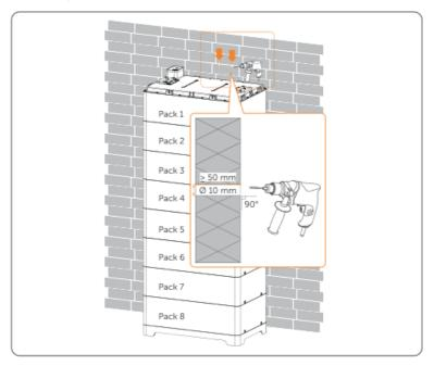
Figure 7-11 Drilling holes
