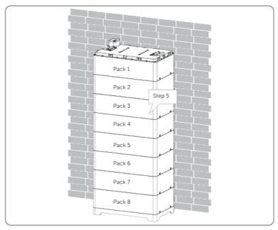
Figure 7-8 Placing battery pack
