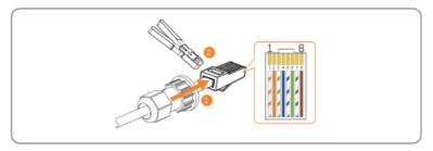
Figure 7-24 Crimping RJ45
