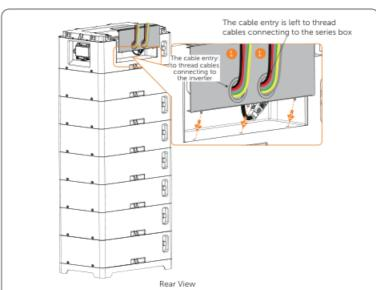
Step 9: Insert such cover into holes on the BMS.
