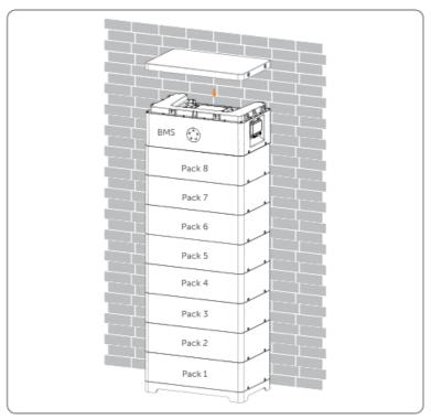
Figure 6-34 Placing BMS
