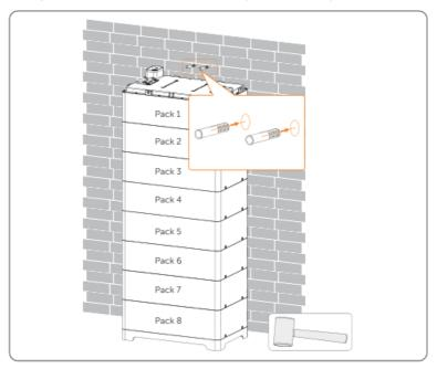
Figure 6-12 Inserting expansion bolt
