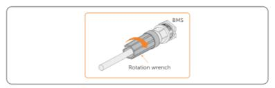
Figure 7-37 Closing communication cable
