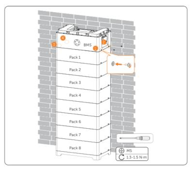
Figure 7-15 Tightening M5 screw
