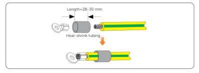
Figure 7-19 Cutting heat-shrink tubing
