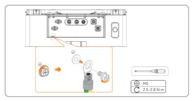
Figure 6-20 Tightening M5 screw
