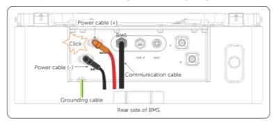
Figure 7-31 Connecting cables to inverter
