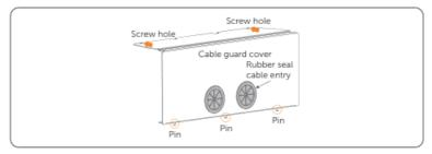
Figure 7-29 Details of cable guard cover
