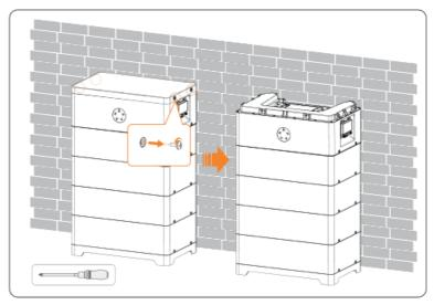
Figure 9-3 Removing BMS cover
