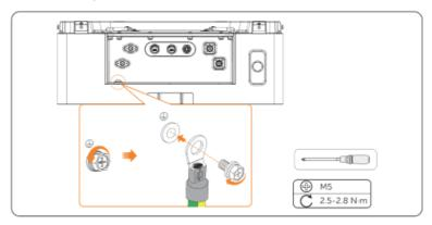
Figure 7-21 Tightening M5 screw
