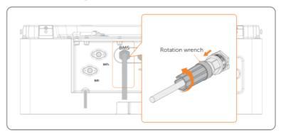
Figure 9-8 Unplugging communication cable
