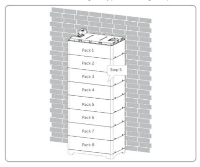
Figure 6-8 Placing battery pack
