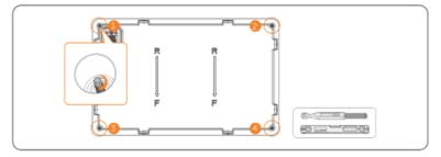
Figure 6-4 Rotating adjustable screw
