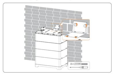
Figure 9-11 Removing assembled bracket
