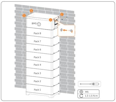
Figure 6-35 Tightening M5 screw
