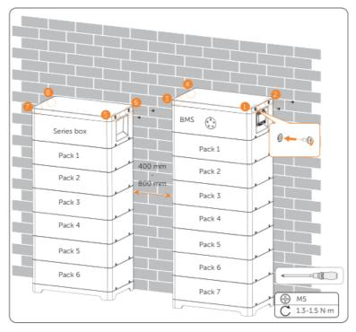
Figure 7-43 Tightening M5 screw
