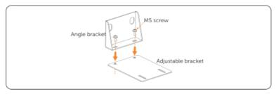
Figure 6-9 Assembling bracket
