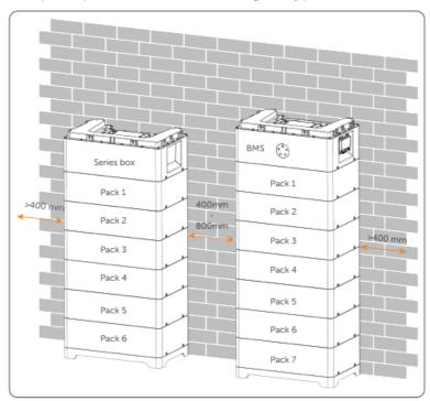
Step 13: Repeat steps 1 to 12 to install the remaining battery packs and series box.
