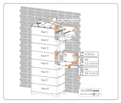
Figure 7-13 Securing assembled bracket
