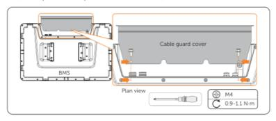
Figure 6-32 Tightening M4 screw
