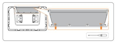
Figure 9-4 Removing cable guard cover
