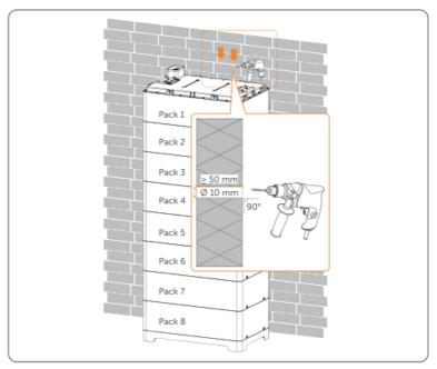
Figure 6-11 Drilling holes
