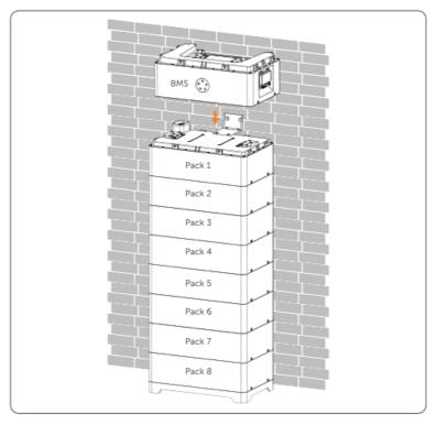
Figure 6-14 Placing BMS
