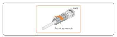
Figure 7-32 Closing communication cable
