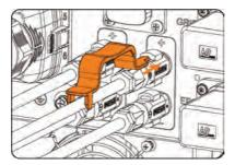
Figure 13-4 Removing the Battery connector
