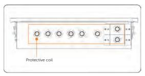
Figure 15-25 Removing the protective coil
