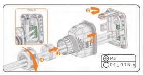
Figure 8-65 Connecting to the inverter
