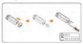
Figure 8-68 Assembling the dongle
