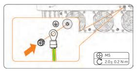
Figure 8-7 Securing the PE cable
