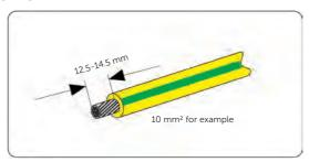
Figure 8-3 Striping the PE cable
