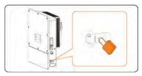
Figure 15-39 Installing the locks
