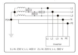
Figure 2-4 Supported power grid-TN-C-S
