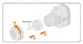
Figure 8-43 Disassembling the connector
