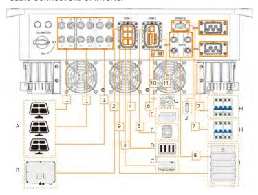
Figure 8-2 Cable connections of inverter
