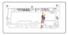
Figure 15-32 Connecting the battery power cable
