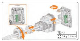
Figure 8-62 Connecting to the inverter
