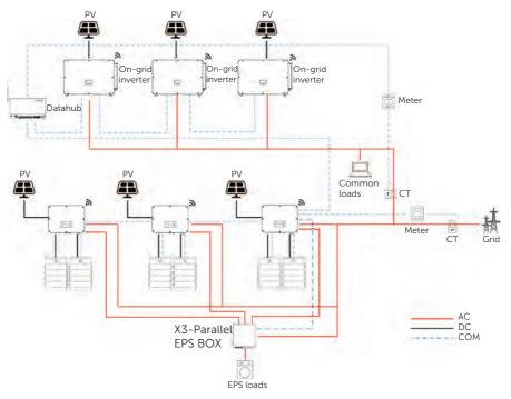
Figure 15-10 DataHub wiring diagram
