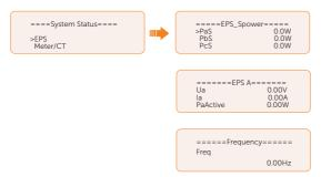
Meter/CT status: Information contains feed-in power of L1, L2 and L3 detected by the connected meter or CT. Positive represents feeding electricity to the grid, negative represents drawing electricity from the grid (buying electricity).
