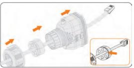
Figure 8-54 Threading the cables
