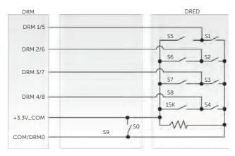
Figure 8-46 DRED wiring diagram
