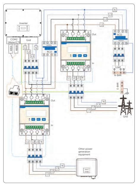
Figure 8-49 Meter connection diagram 2
