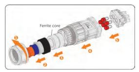
Figure 8-9 Disassembling the AC connector
