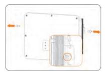
Figure 13-8 Unscrewing the M5 screws
