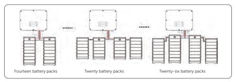
Figure 8-25 Battery connection Scheme 2
