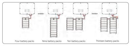
Figure 8-27 Battery connection Scheme 3
