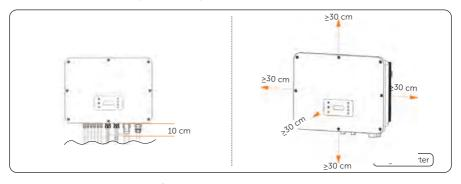
Figure 5-4 Clearance requirement for single inverter
