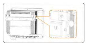
Figure 7-11 Locking the inverter
