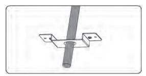
Figure 15-29 Threading the cable
