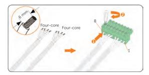
Figure 8-61 Connecting to 8-pin terminal block
