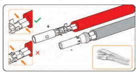
Figure 8-17 Crimping the terminal
