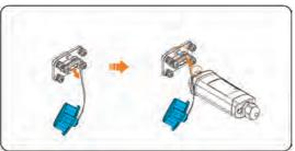
Figure 8-69 Wi-Fi connection procedure
