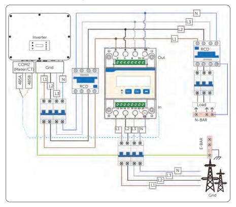
Figure 8-48 Meter connection diagram 1
