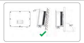
Figure 7-1 Correct installation
