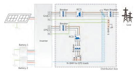
Figure 2-11 Application scheme for X3-ULT-10K / 15K-GLV
