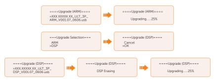
After the upgrade is completed, the LCD screen displays Upgrade Successful. If the upgrades fail, the LCD screen displays Upgrade failed.
