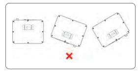
Figure 7-2 Incorrect installation
