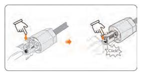
Figure 8-32 Press down on the Spring
