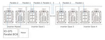
Figure 15-21 Communication connection with X3-PBOX
