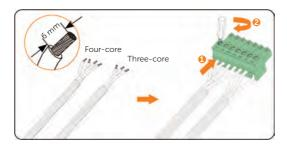
Figure 8-64 Connecting to 7-pin terminal block
