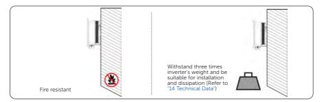
Figure 5-3 Installation carrier requirement
