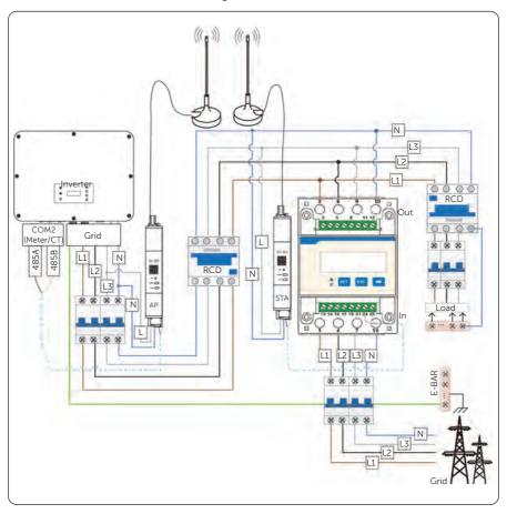
Figure 8-50 Wireless Meter connection diagram
