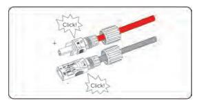
Figure 8-19 Securing the PV cable
