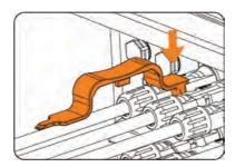
Figure 13-2 Releasing the PV connector
