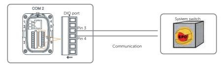
Figure 8-63 System switch connection diagram
