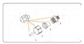
Figure 8-70 Disassembling the waterproof connector
