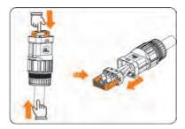
Figure 13-7 Disconnect the AC connector
