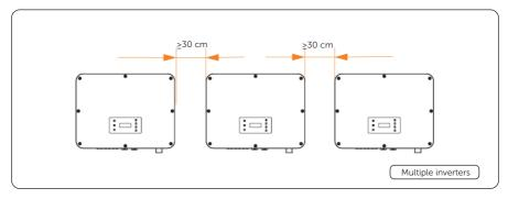
Figure 5-5 Clearance requirement for multiple inverter
