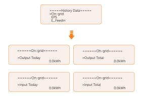
EPS: A record of the output electric energy of the inverter today and the total.
