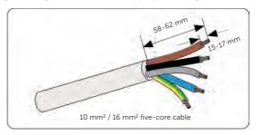
Figure 8-8 Stripping the Grid cable
