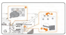
Figure 15-34 Installing the WiFi connecting cable
