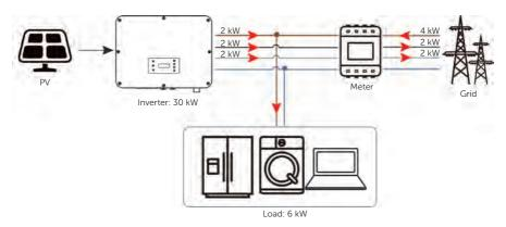
Figure 2-17 Zero export control with Phase Unbalance disabled
