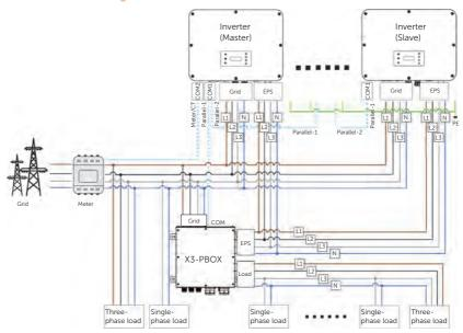
Figure 15-17 System diagram with SolaX X3-PBOX
