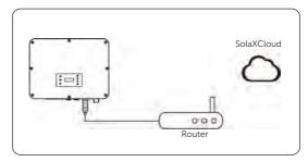
Figure 8-67 LAN mode connection diagram
