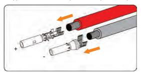
Figure 8-16 Inserting the PV pin contact
