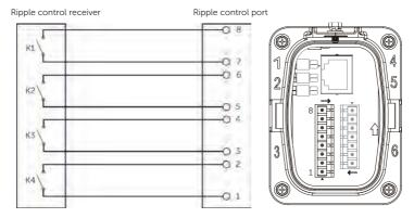
Figure 8-58 Connection diagram for ripple control
