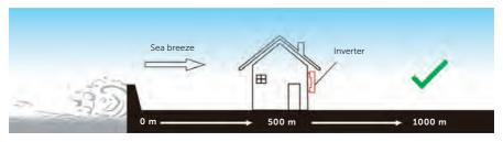
Figure 5-1 Recommended installation position
