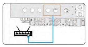
Figure 15-37 Installing the dongle
