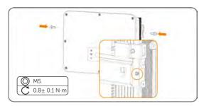
Figure 7-10 Securing the inverter
