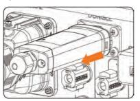
Figure 13-3 Removing the dongle
