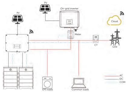
Figure 15-13 Micro-grid wiring connection
