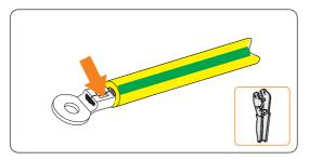
Figure 8-5 Crimping the cable
