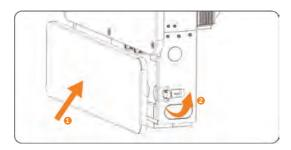
Figure 15-38 Installing the front panel
