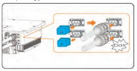
Figure 8-13 Installing the AC connector to inverter
