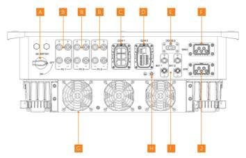
Figure 8-1 Terminals and Ports of Inverter
