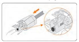
Figure 8-31 Threading the battery cable
