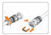
Figure 13-6 Remove the swivel nut
