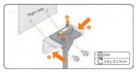
Figure 15-35 Installing the WiFi stand
