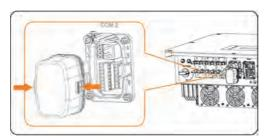
Figure 8-52 Disassembling the COM 2 port
