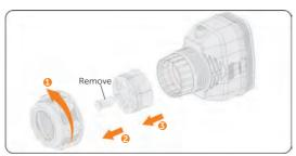
Figure 8-53 Disassembling the connector
