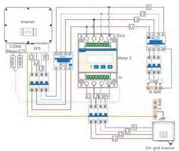
Figure 15-16 Connection diagram of Meter on EPS port
