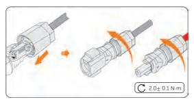
Figure 8-33 Tighten the cable gland
