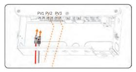
Figure 15-31 Connecting the PV cable
