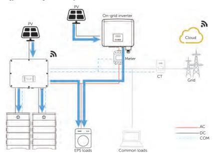
Figure 15-15 Power flowing when grid off
