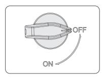
Figure 13-1 Turning off the DC switch
