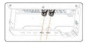
Figure 15-33 Connecting to COM port
