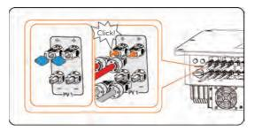
Figure 8-21 Connecting the PV cable
