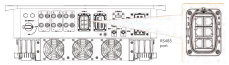
Figure 15-8 Connection port for EV-Charger
