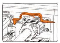
Figure 13-5 Removing AC connector
