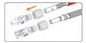
Figure 8-18 Threading the PV cable
