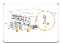
Figure 12-1 Disconnect the fans connectors
