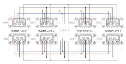
Figure 15-19 Power cable connection with X3-PBOX
