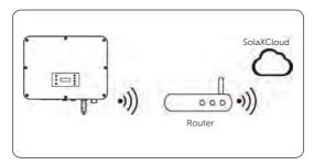
Figure 8-66 Wi-Fi mode connection diagram
