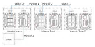
Figure 15-22 Communication connection without X3-PBOX
