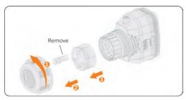
Figure 8-60 Disassembling the connector
