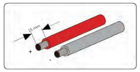
Figure 8-29 Striping the battery cable
