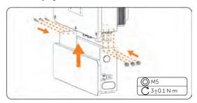
Figure 15-24 Installing the cable cover
