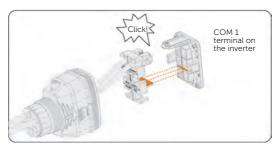
Figure 8-39 Inserting the connector to COM 1
