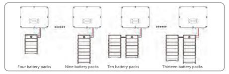
Figure 8-23 Battery connection Scheme 1
