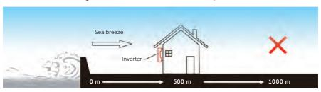
Figure 5-2 Incorrect installation position
