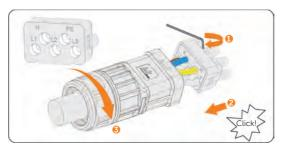
Figure 8-12 Assembling the AC connector
