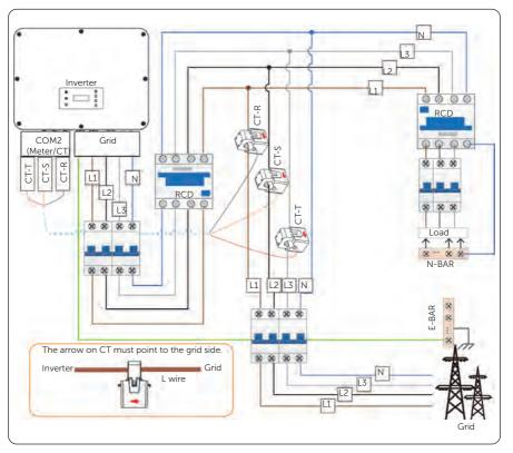
Figure 8-51 CT connection diagram
