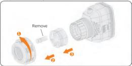
Figure 8-36 Disassembling the connector
