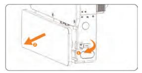
Figure 15-26 Removing the front panel
