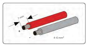
Figure 8-15 Striping the PV cable
