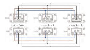
Figure 15-20 Power cable connection without X3-PBOX
