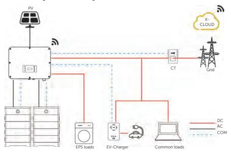
Figure 15-7 EV-Charger wiring diagram
