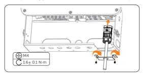
Figure 15-30 Installing the AC connector
