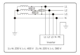
Figure 2-2 Supported power grid-TT
