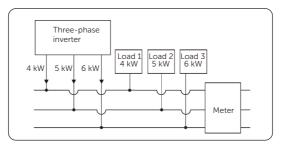
Figure 10-7 Phase Unbalanced enabled
