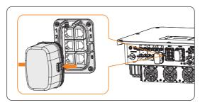
Figure 8-35 Removing the connector enclosure
