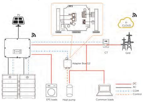
Figure 15-4 Adapter Box G2 wiring diagram
