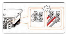
Figure 8-34 Connecting the battery connector
