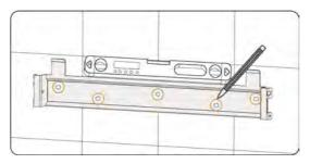
Figure 7-5 Marking the holes
