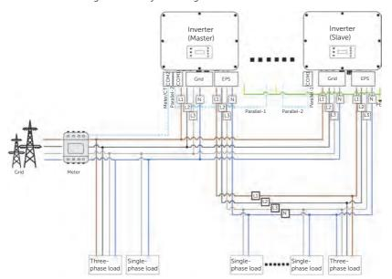
Figure 15-18 System diagram without SolaX X3-PBOX
