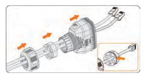
Figure 8-37 Threading the cables
