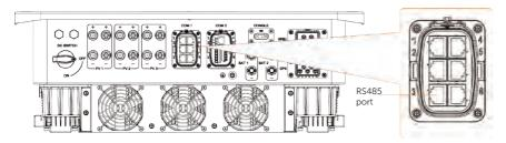
Figure 15-11 Connection port for DataHub
