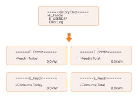
E\_USERDEF: The electricity of the connected on-grid inverter today and the total.(detected by Meter 2) This function is only available when the meter 2 is connected.
