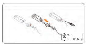
Figure 8-71 Assembling the dongle
