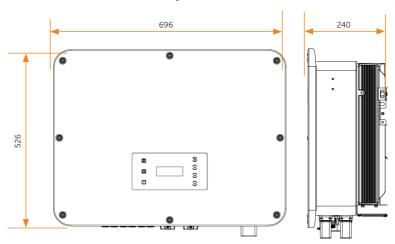
Figure 7-3 Dimensions 1 (Unit: mm)
