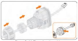
Figure 8-44 Threading the cables
