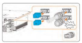
Figure 8-14 The EPS port is not connected
