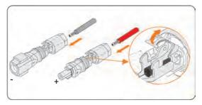
Figure 8-30 Opening the spring
