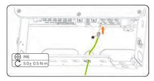
Figure 15-27 Connecting the PE cable
