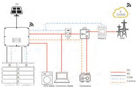
Figure 15-2 Dry contact wiring diagram
