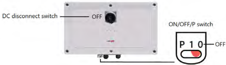
ON/OFF/P and DC disconnect switches
