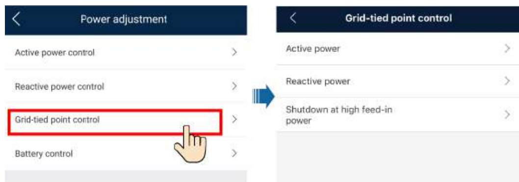
Figure 7-10 Grid-tied point control
