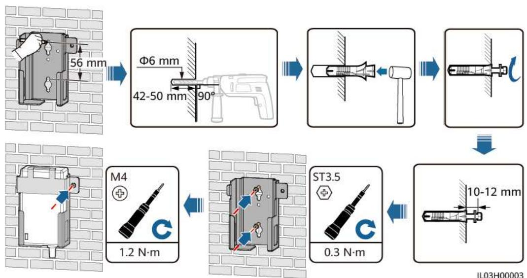
Figure 3-10 Wall-mounted installation (mode 2)
