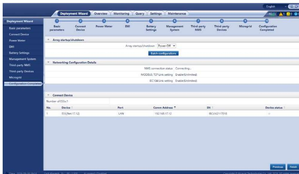
**Step 11** (Optional) Perform wire sequence detection. This function applies only to the LUNA2000-215-2S10, LUNA2000-215-2S11, LUNA2000-215-2S12, LUNA2000-161-2S11, and LUNA2000-107-1S11 C&I liquid-cooled ESSs, and is displayed in multi-ESS scenarios. Tap **Starting up** to start wire sequence detection.
