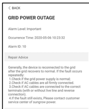
figure 7-9 Detailed Fault Alarm Information
