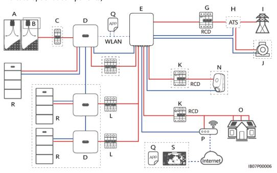
**Figure 2-6** Networking with some of loads connected to the SmartGuard (dashed boxes indicate optional components)
