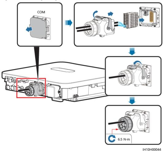
Figure 5-34 Securing the signal cable connector
