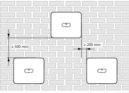
Figure 4-4 Triangle installation mode (recommended)
