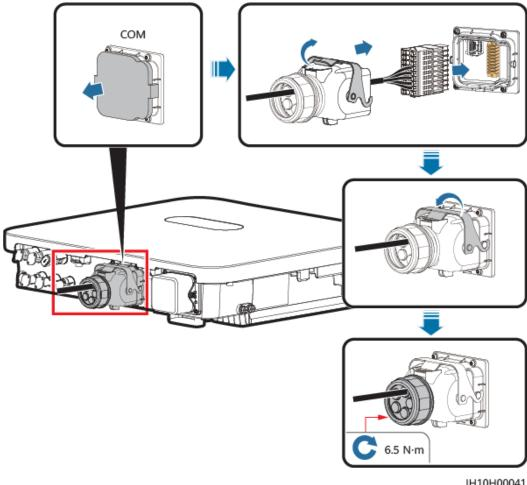
Figure 5-37 Securing the signal cable connector
