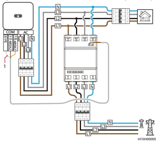
Figure 5-25 Three-phase, four-wire direct connection (Smart Dongle networking)
