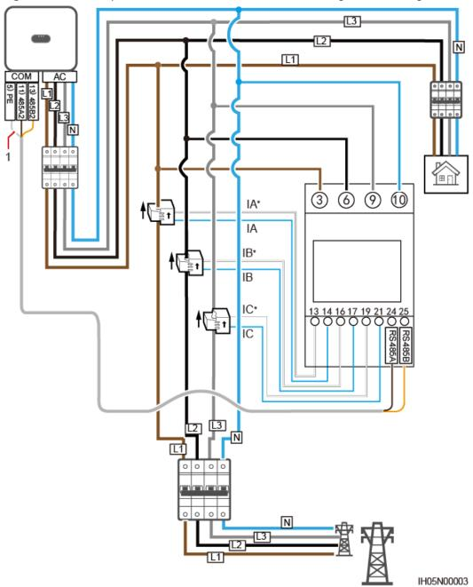
Figure 5-23 Three-phase, four-wire connection (Smart Dongle networking)
