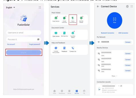
Figure C-1 Method 1: mobile phone connected to the Internet
