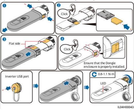
Figure 5-45 Installing the 4G Smart Dongle (SDongleB-06)
