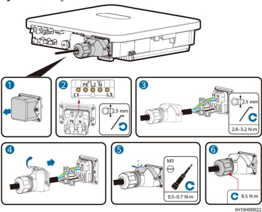
Figure 5-5 Securing the AC connector
