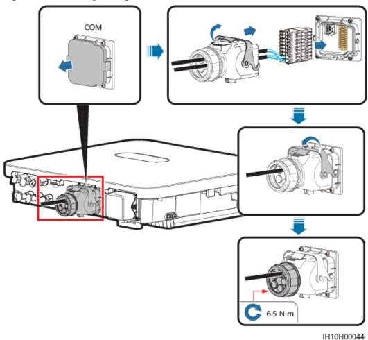
Figure 5-40 Securing the signal cable connector
