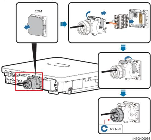
Figure 5-27 Securing the signal cable connector
