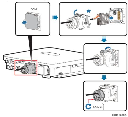
Figure 5-20 Securing the signal cable connector
