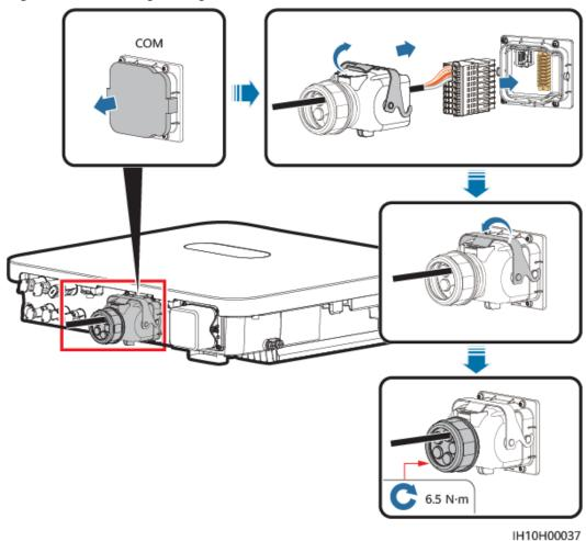
Figure 5-29 Securing the signal cable connector
