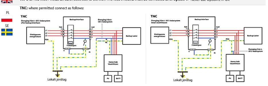
TN-C-S: Use Option 2, if only the phase conductors may be disconnected in island operation. TT/TN-S: Use Option 1, if the neutral conductor (N) is required to be connected to the protective earth conductor (PE) in island operation (star point simulation).
