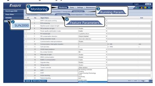
Figure 6-50 Setting tracking system controller
