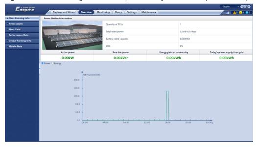
Figure 6-4 Plant running information (with battery but without power meter)
