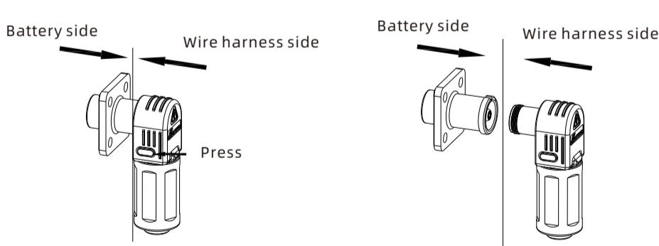
Press the position indicated in the figure above before disconnecting the power terminal.
