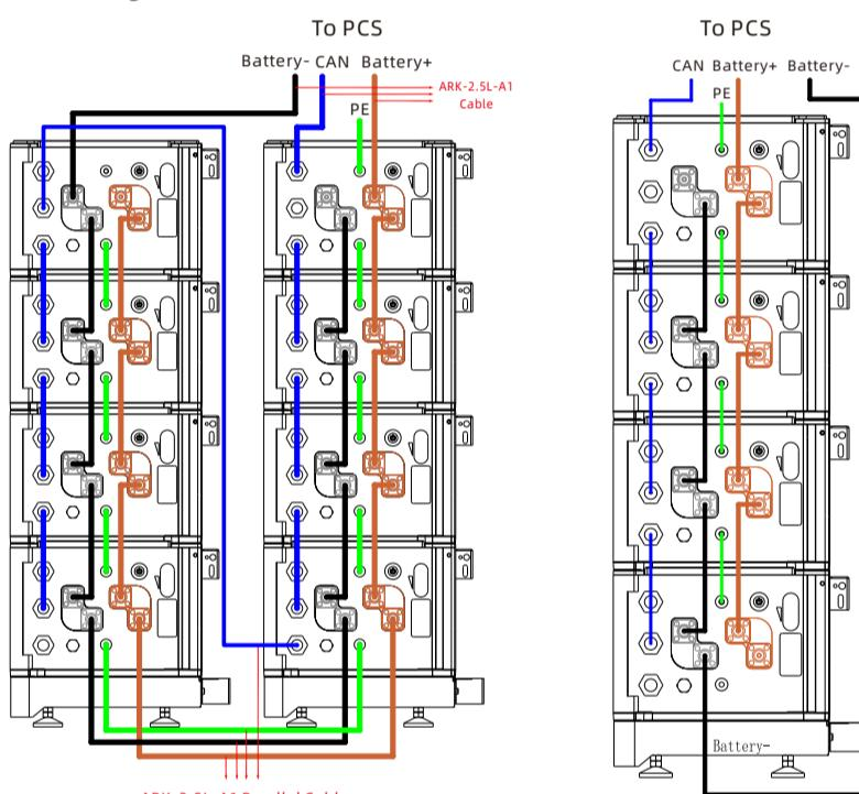
**Note:** The switch connect PCS to ARK-2.5L-A1, we recommend the use of molded case circuit breaker with rated working voltage greater than 125V and rated working current greater than 125A.
