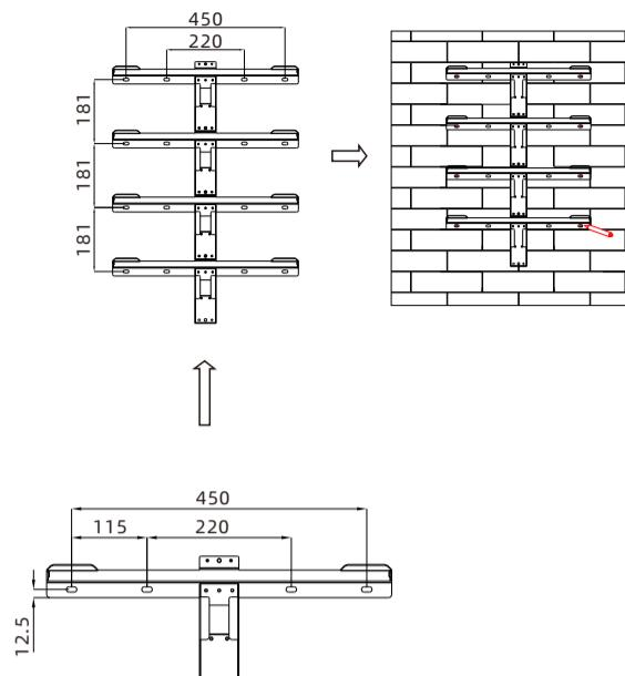
**Note:** Avoid drilling holes in the water pipes and cables buried in the wall.
