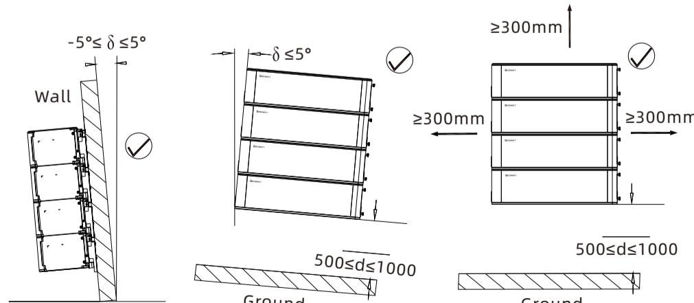
**Note:** The number of wall-mount installations should not exceed four. Please make sure that the weight capacity of wall should exceed 150kg.
