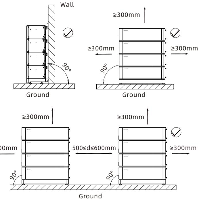
1. If more than 4 batteries are used, base mounting is recommended.
