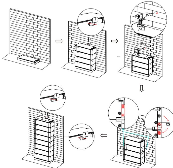
**Note:** The safety part needs to be installed at the top battery, however, once the number of the battery pack is higher than 7, one more safety part should be installed in the middle battery which is shown the last step. Avoid drilling holes in the water pipes and cables buried in the wall.
