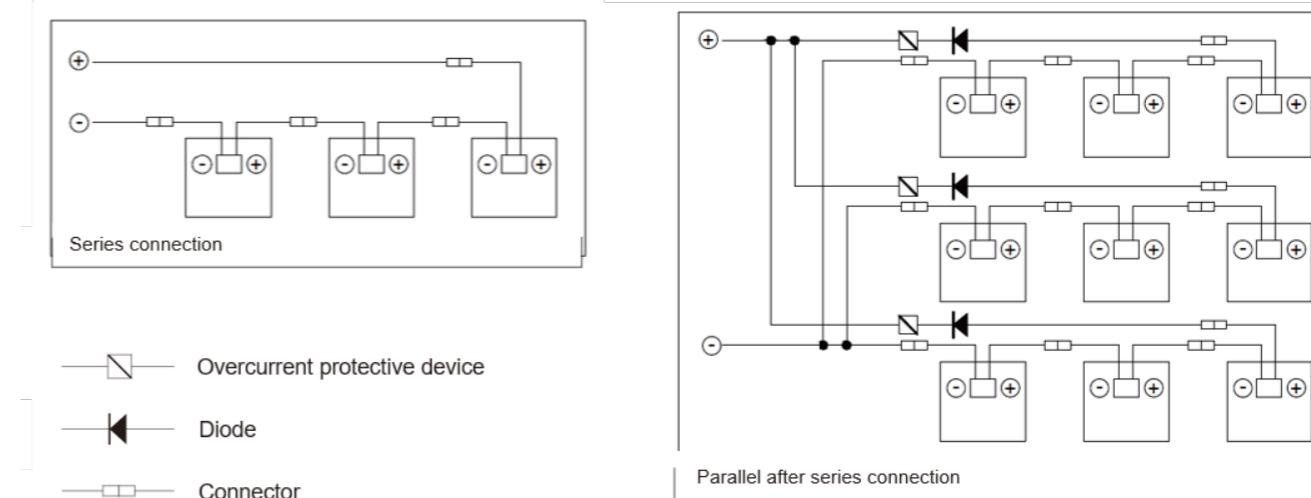
If the PV module is passed through by a reverse current greater than the maximum fuse current of the PV module, the PV module shall be protected with an over current protector of the same specification. If more than two strings are connected in parallel, each PV module string shall be protected with an over current protector as shown above.
