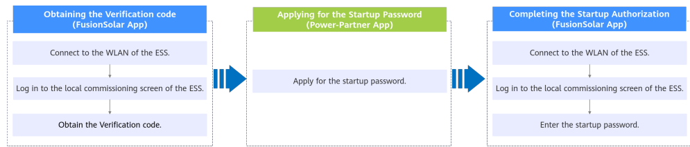
Figure 9-2 ESS startup authorization procedure
