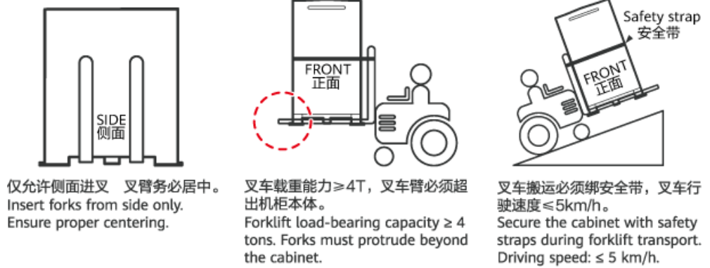
Figure 3-1 Loading and unloading requirements
