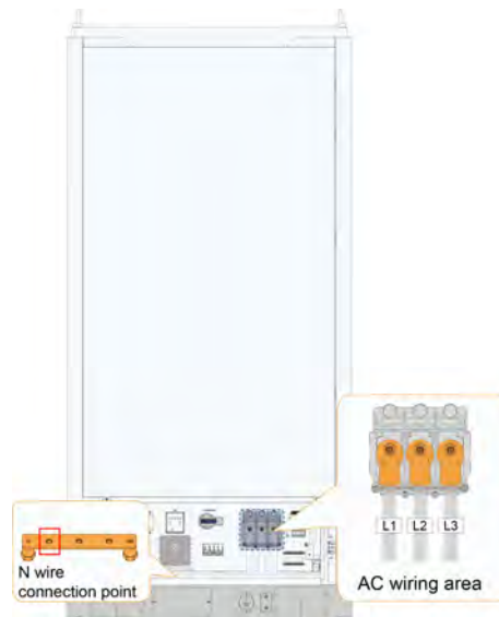
Figure 5-9 AC Wiring Area
