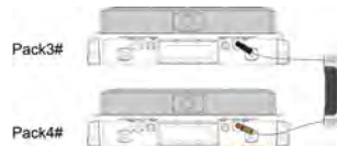
Figure 6-3 Insert Fuse Plugs into PACK Bases
