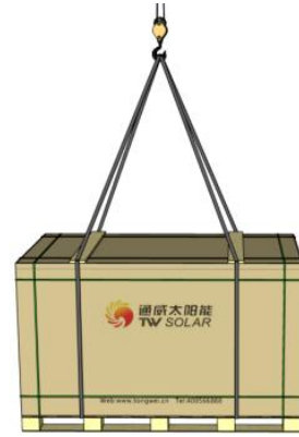
Figure 6 Schematic diagram of Module lifting
