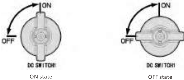
Fig 9.8 DC switch status
