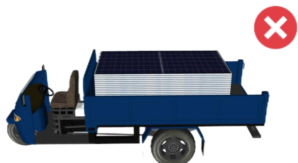
Figure 9 Do not use a tricycle to transport the Module
