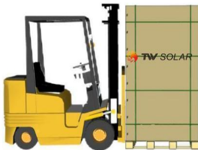
Figure 6 Please note the protection of Module and forks
